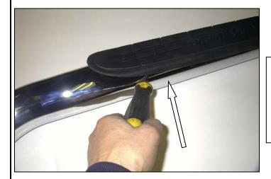
**Step-2** Working from the back of the step pad position a flat blade screw driver underneath the step pad and pry upward to remove from the tube.
