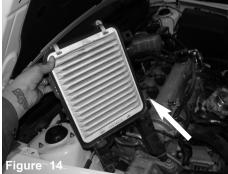
Carefully manuever the bottom half of air box out of vehicle. Note: becarefull and not damage the A/C line. Re-install the bolt from previous step and secure the A/C line.
