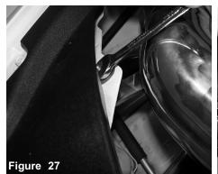
Tighten both nuts on vibra mount using 10mm
