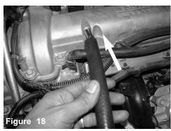
Attach the provided 10mm hose to the engine.
