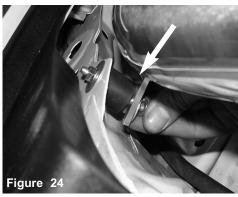
Secure the bracket on intake tube using provided M6 washer and nut.
