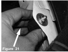
Secure the vibra mount using M6 nut and washer.
