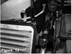
With 10mm socket and ratchet, loosen and remove the bolt holding in A/C line and air box.
