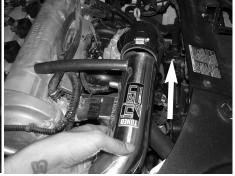
Install the intake asembly into the vehicle and position to hose.
