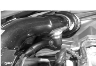
Install the high flow filter to intake tube and tighten using 8mm nut driver Make sure everything is tighten. Position for best possible fit. Tighten all clamps using 8mm nut driver.
