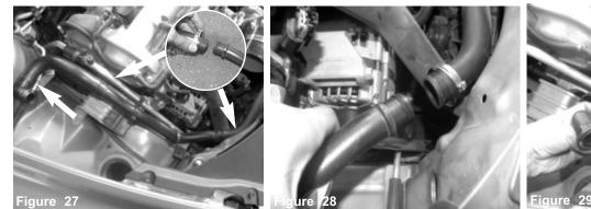
Remove the plastic hard line from the vehicle.
