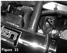
Connect crank case line to intake tube.
