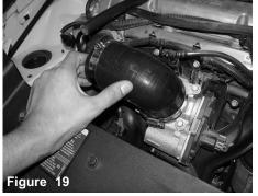
Install the elbow hose with clamps provided to the throttle body. *Make sure the short side of hose is on the throttle body.*
