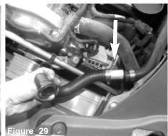
With plastic hard line removed, connect the 2 soft lines together using provided coupler. Position for best fit.
