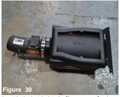
Insert the intake tube into the filter on power flow box as shown above. The assembled air intake and power box is ready to be installed. Tighten clamp on filter using 8mm nut driver.
