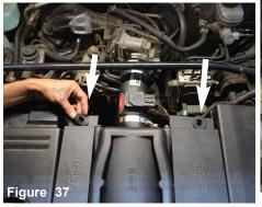
The stock grommet are removed from the stock air box and inserted into the pre-drilled holes on the top air panels.
