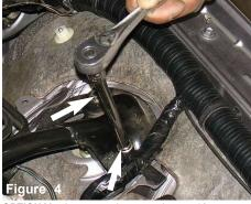
**OPTIONAL:** Loosen and remove the two 12mm nuts located on the each strut tower mount. Once you have removed all four 12mm nuts, continue to removed the strut tower bar.
