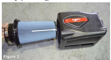
Install the provided Twist lock filter into the PowerFlow
