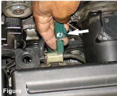
Depress the tab on the green electrical clip and pull the clip from the vacuum switching valve. **Note:** on automatic transmissions, skip step and go to figure 8.
