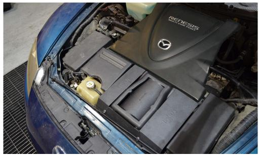
Align the entire intake for best possible fit. Once you have aligned and made sure that the length of the intake is free from any moving parts, continue to tighten all nuts, bolts and clamps. Congratulations! You have just completed the installation of this intake system. Periodically, check the alignment of the intake, normal wear and tear can cause nuts and bolts to come loose. Failure to check the alignment and adjust the intake can cause damage that will void the warrantv.
