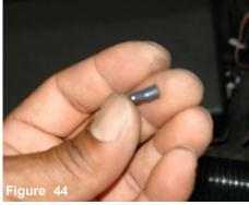
The 5mm vacuum cap is used to cap off the intake manifold port.
