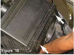
Unlatch the metal clamps on the lower air box cleaner. Once you have removed the clamps, continue to pull the upper air box from the lower air box.
