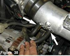
The two lower vacuums lines are pressed over the lower intake ports as shown above.
