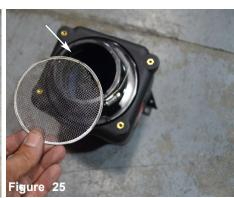
Now install the 3-3/4 metal screen into the filter
