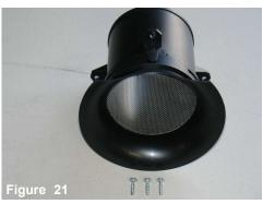
Here is the air horn and three screws that have been removed from the lower air box cleaner.
