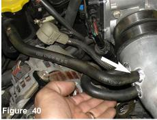
The upper vacuum hose is installed on the upper intake port. NOTE: Some models may only have 2 vacuum lines. The supplied 8mm vacuum cap will be used to cap off the extra port on the intake tube.
