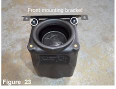
With provided M6X12 socket cap screws secure the front mounting bracket to the top of the power flow
