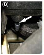
The vacuum line leading from the air box canister to the intake manifold port is removed (A). The vacuum cap supplied is used to cap off manifold port (B). Note: The canister will be removed for this application. For automatic transmisions go to figure 17.
