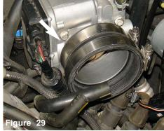
Install the step hose with clamps provided. Tighten the clamp on the throttle body side.
