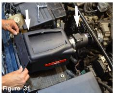
The assembled power box is lowered into the engine compartment and the intake is pressed into the throttle body step hose.
