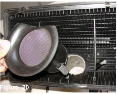
Once all three screws have removed, continue to remove the air horn from the air box.
