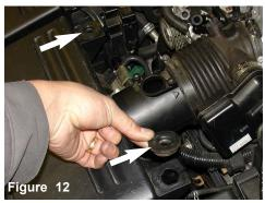
Remove the stock grommets from the air box cleaner. To be used later in the instructions.
