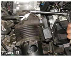
Loosen the clamp on the throttle body air hose as shown above.
