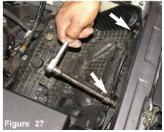
The lower air box nuts are loosened and removed in order to place the new power box. The first nut is now removed
