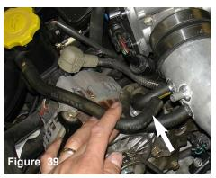
The upper vacuum hose is aligned to the upper intake port. NOTE: Some models may only have 2 vacuum lines. The supplied 8mm vacuum cap will be used to cap off the extra port on the intake tube.
