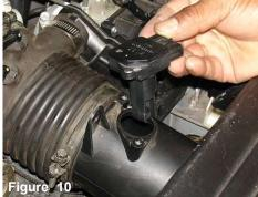
Once both screws have been removed, continue to pull the mass air flow sensor from the sensor housing.
