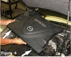
pull up on the stand offs located in front of the engine cover. A slight tug up will be required to pull the stand offs out of the stock grommet.
