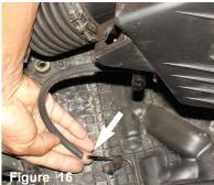
The vacuum line leading from the air box vacuum switching valve is disconnected from the hard line found under the air box. A 5mm vacuum cap is used to cap the hard line
