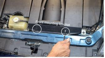
Secure the front of the panels using provided M6X20 button head screws. Secure and tighten all screws on both sides of the panels.
