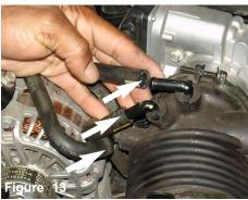
All three vacuum lines are disconnected from the air intake duct connected to the throttle body. **Note:**Some models only have two vacuum lines.
