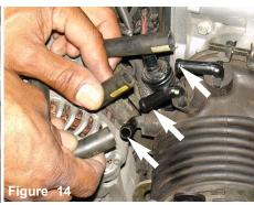
All three vacuum lines have been disconnected from the air intake duct.
