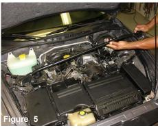
All four 12mm nuts have been removed and the strut tower bar is now pulled out.
