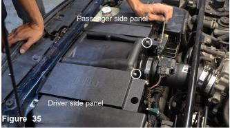
Place the passenger side and driver side panel on top and secure to the back of the power flow box using provided M6X12 socket cap screws.
