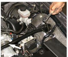
The strut tower bar is replaced to stock position. Use a socket and ratchet to fasten the flange nuts over the strut tower bar.
