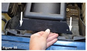
The front mounting panel tabs are aligned to the studs as shown above.
