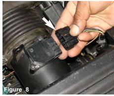
Disconnect the electrical sensor harness from the mass air flow sensor.
