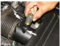
Unscrew and remove the two screws that fastens the mass air flow sensor to the sensor housing.
