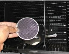
Remove the 3 3/4 " OD metal screen from the lower air box as shown above. Save for later install.
