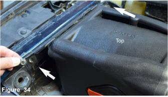
The stock nuts are used to fasten the mounting panel to the crossmember radiator support. Use a ratchet and socket to tighten the nut on the passenger and driver side front mounting panel. Secure and tighten.
