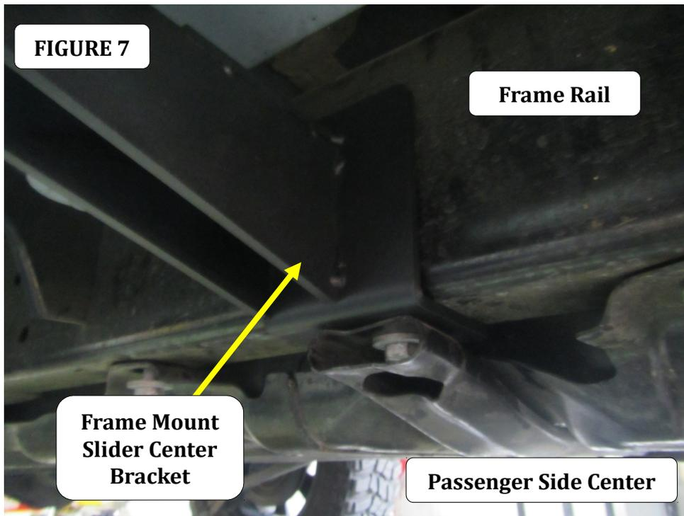
**Step-7** Position the rear bracket between the frame rail and the skid plate by pulling down gently the skid plate using a flat screwdriver . Secure using the bolt removed. Figure 8. Leave the bolt loose for final adjustment.
