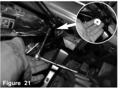
Secure the bracket to the vibramount using provided m6 nut and fender washer. Do not tighten.
