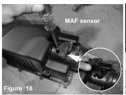
With Phillips screwdriver, loosen the 2 screws holding in the MAF sensor. Remove the MAF sensor from the stock intake tube.
