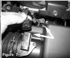
Disconnect the MAF sensor harness. pull clip harness away from the air box.
