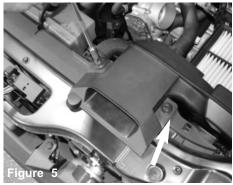
Loosen and remove the 2 bolts holding in the factory scoop.
