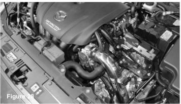
Congratulations! You have just completed the installation of this intake system. Periodically, check the alignment of the intake, normal wear and tear can cause nuts and bolts to come loose. <u>Note: Check clearance and adjust if needed! Failure to check the alignment and adjust the intake can cause damage that will void the warranty. Injen Technology is not responsible for any damages caused by/from improper installation.</u>
