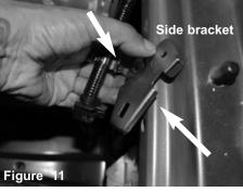
Pull back the harness from the bracket, remove the bracket from the vehicle.
