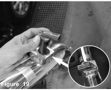
Install the MAF sensor into the intake tube and secure using provided M4 screws. Tighten using 2.5mm allen key.
