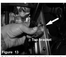
Pull back the harness from the bracket, remove the bracket from the vehicle. .
