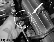
Locate the harness bracket that is located on the side of the vehicle frame. Remove using 10mm socket and ratchet.
