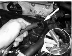
Install the provided new crank case 10mm hose and secure on engine and intake side.
