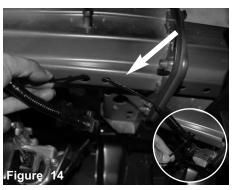
Locate the 2 holes that are on the frame. Run the provided zip-tie like above image. Make sure harness is moved over allowing for New Injen intake installation.
