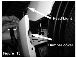
Loosen the screws and pull back the bumper cover on driver side, this will allow filter installation. Loosen the screws on side and bottom of the splash guard also. This will allow for filter installation.
