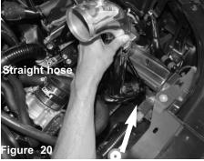
Install the straight hose with clamps to the throttle body. Install the intake tube in to vehicle and position the tube to staight hose and bracket to vibramount from step 17.
