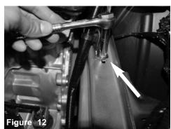
Locate the last harness bracket on top of the vehicle frame. Remove using 10mm socket and ratchet.
