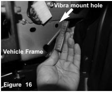
With provided trim-seal, attach to the lip that is on the vehicle frame. This will prevent any contact with the intake and frame. Take note of hole that will be used for the vibramount.
