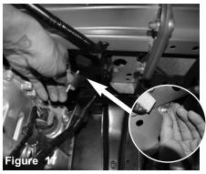
From the inside of the engine compartment, locate the hole from the previous step, and secure from the other side using provided M6 nut and fender washer.
