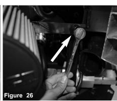
Position for the best possible fit and clearance . Secure the bracket and tighten using 10mm socket and ratchet.
