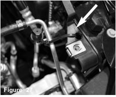
With provided zip-tie, secure the A/C line to the front core support hole. Note: Injen Technology is not responsible or liable for damage to A/C line or intake system and will not be covered under warranty for inproper installation or clearance issues.
