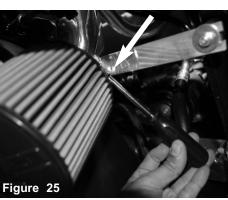
Secure and tighten using 8mm nut driver.
