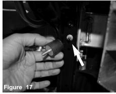
Locate the 2nd thredded fitting closes to the bottom of the frame. Attach the Male/female vibramount to the fitting.
