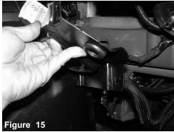
Remove the air box bracket.
