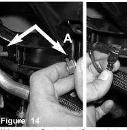
A) Loosen the 2 nuts using 13mm socket or wrench holding in the air box bracket.
