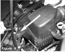
Loosen the bolt holding in the air box using 10mm socketa
