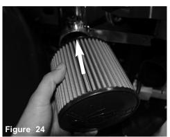
Install the filter to the tube.
