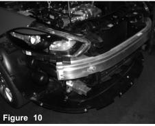
Remove the front bumper cover. Loosen and remove clips and screws on top, side and bottom of cover. Carefully remove the cover.
