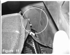
Carefully pull back clip located on the radiator splash guard holding in the resonator scoop, loosen the screw on splash guard using 10mm socket or wrench.
