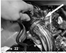
Position for the best fit and tighten the clamp on the
