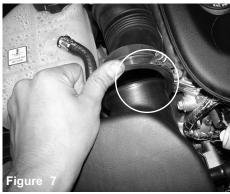
Loosen the clamp on the air box using 8mm nut driver, loosen and pull back.
