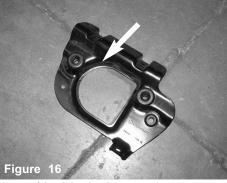
Image of the air box bracket removed.
