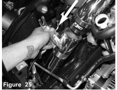
Now install the lower part of the intake assembly into the vehicle, position to the upper intake assembly and bracket to the vibra mount. Secure the bracket using provided fender washer and nut.
