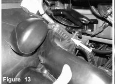
Now remove the resonator scoop from the air box bracket.
