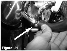
Now secure the crank case line to the fitting.
