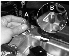
A)Now install the vibra mount to the thredded fitting. B)Now secure and tighten the fitting.
