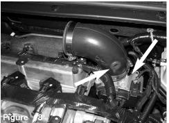
Now install the elbow hose with clamps provided to the throttle body, make sure the side with the grommet is closer to the throttle body.
