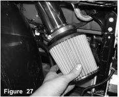
Install the air filter to the lower intake assembly and tighten using 8mm nut driver.
