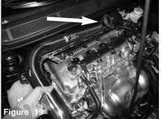
Install the intake tube into the elbow, and position the bracket to the vibra mount.
