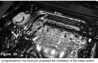
Congratulations! You have just completed the installation of this intake system. Periodically, check the alignment of the intake, normal wear and tear can cause nuts and bolts to come loose. <u>Note: Check clearance and adjust if needed!</u> <u>Failure to check the alignment and adjust the intake can cause damage that will void the warranty. Injen Technology is not responsible for any damages caused by/from improper installation.</u>
