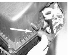
Pull back the crank case line from the air box.
