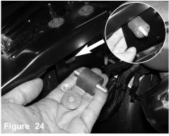
Install the vibramount with fender washer and nut, secure and tighten the back to the radiator support frame.
