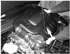
Lift up and remove the engine cover/air box assembly out of the vehicle.
