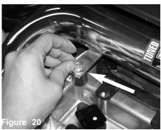
Now secure the bracket using provided M6 nut and washer.
