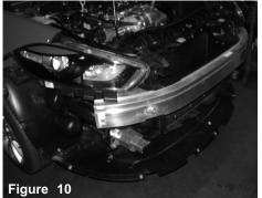
Remove the front bumper cover. Loosen and remove clips and screws on top, side and bottom of cover. Carefully remove the cover.
