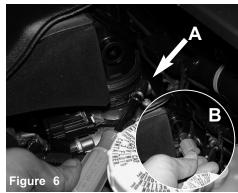
A) Loosen the clamp on the throttle body. B) Loosen and remove the
