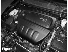
Stock box shown in this picture. Remove engine cover. Disconnect negative battery terminal.
