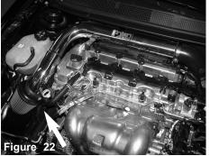
Now install the filter to the intake tube for the short ram position and tighten using 8mm nut driver. Tighten all clamps and secure the vibra mount and tighten using 10mm socket and ratchet.
