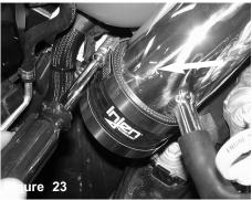
For cold air application, remove the air filter and install the provided 3" hose with clamps to the upper intake assembly. Tighten on the tube only.
