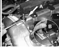
A)Loosen the fitting on top of the valve cover using 13mm wrench. B)Remove the fitting.
