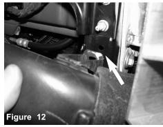
Remove the clips holding in the resonator scoop on vehicle frame.
