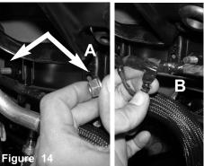
A) Loosen the 2 nuts using 13mm socket or wrench holding in the air box bracket.B) Pull back any lines that are attached to the air box bracket.
