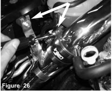
Position for the best possible fit and clearance and tighten the clamps using 8mm nut driver. Secure the bracket and tighten using 10mm socket and ratchet.
