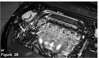
Re-position if necessary and tighten if needed. Make sure there is enough clearance. Re-install the bumper cover and connect the battery terminals.
