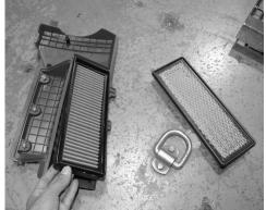
Loosen the 3 bolts holding in the upper air box. Remove the old paper filter and replace with the new injen flat panel filter. Re-install and secure.
