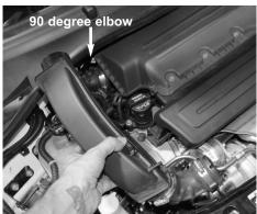
Loosen clamp on turbo. Loosen clamp on the 90 elbow. Disconnect the vacuum line using pliers. Remove the factory intake tube.
