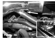
Connect the crankcase line to fitting on intake tube and secure Tighten and secure the intake tube using 8mm nut driver
