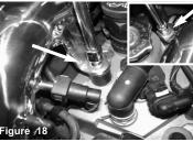
Secure and tighten both brackets on intake tube using pro- Install the filter to the intake tube and tighten using 8mm vided fender washers and nuts. Tighten using 10mm sock- nut driver. et and ratchet.
