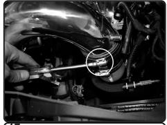
17. Secure the hose and tighten clamps using 8mm nut driver.
