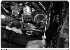
11. Tighten the clamp on turbo only.
