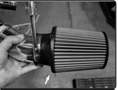
**13.** Secure and tighten using 8mm nut driver.
