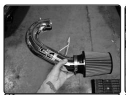
12. Install the filter to the tube.
