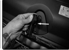
**7.** Carefully remove the lever out of vehicle,
