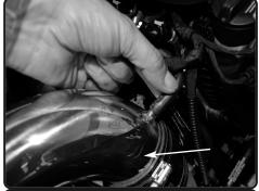
**18.** Connect the vacuum line to the fitting on the intake tube.
