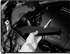
**5.** Remove the ram scoop from vehicle.
