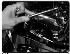
**16.** Tighten bracket using 10mm socket or wrench.
