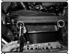
**4.** Locate the 2 bolts holding in the front air scoop and loosen and remove using T25 torx bit. Remove the 2 bolts.
