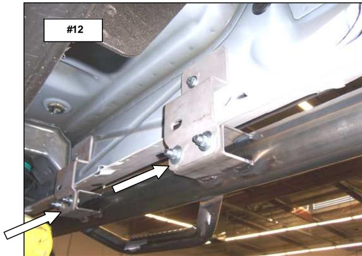
**Step-8** Align the side step with the vehicle and tighten all nuts and bolts.
