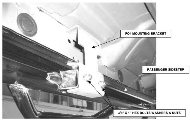
STEP 4. Position the passenger sidestep up to the mounting brackets and loosely attach it to the brackets using the 3/8" x 1" hex bolts, washers and nuts as shown.
