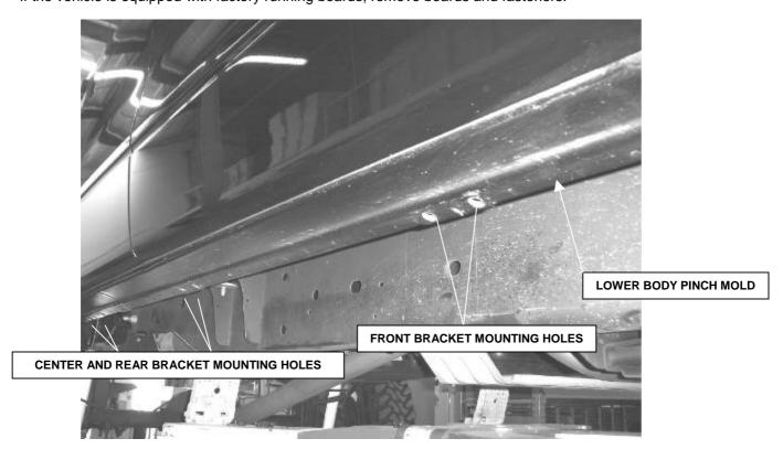
**STEP 2.** This installation uses three mounting brackets per side. Beginning with the passenger side, locate the six holes in the lower body pinch mold.
