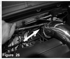
Tighten the clamp on turbo housing using 8mm nut driver.
