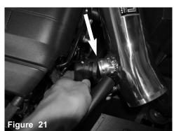
Connect the smog pump line to the machined fitting on intake tube.
