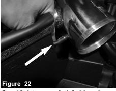
Connect the factory vacuum line to the fitting on the intake tube
