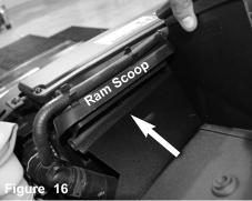
Install the front side with rubber trim underneath the factory Ram scoop first. Position the grommets to the factory OEM air box fittings.
