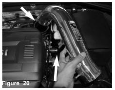
Install the intake tube into vehicle and position the tube to the step hose and bracket to the vibramount.
