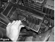
Now, lift up and remove the bottom half of the air box. Complete OEM air box removed.
