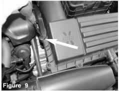
Use a T25 torx bit screwdriver and loosen the upper half of the airbox and remove.
