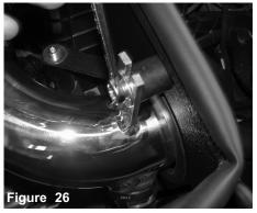
Now secure the bracket using provided washer and nut. Now position the intake tube for the best fit and tighten.
