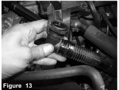
Rotate the smog pump fitting, if equipped, for the position of the new intake.
