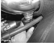
Now connect the smog pump harness to the fitting on the intake tube, if equipped.
