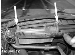
WithT25 torx bit loosen the 2 screws holding in the factory ram scoop and remove. Save screws for later install.
