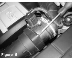
With T25 torx screw, loosen the 2 screws holding in the MAF sensor.
