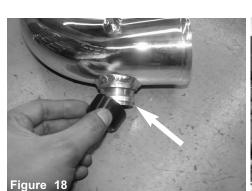
If not equipped with smog pump, cap off using vinyl plug.
