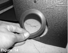
Attach the vinyl trim to the inside of heat shield hole cut out for the intake tube.
