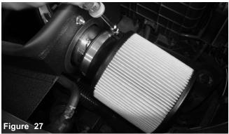
Now install the air filter and tighten using 8mm nut driver. Tighten all clamps using 8mm nut driver. Position for the best fit.
