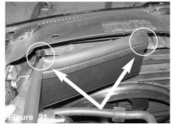
Secure the front of the heat shield using the factory screws. Tighten using T25 torx bit.
