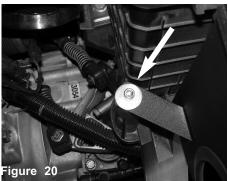
Now secure the tab using provided allen screw and fender washer.
