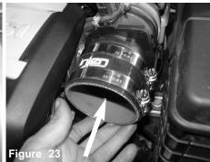
Install the 3-1/8" hose with clamps to the MAF sensor do not tighten.
