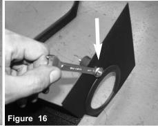
Tighten using 10mm wrench.
