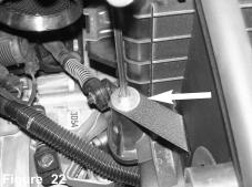
Tighten screw using 6mm allen key.
