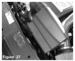
Remove the two T25 torx screws that hold in the factory ram scoop.
