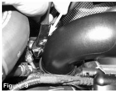
With pliers, pinch the clamp holding in intake tube at the turbo.
