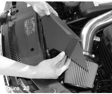
Install the new Injen ram scoop. Position the scoop to factory.
