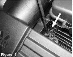
With T30 torx bit, loosen the screw holding in air box.
