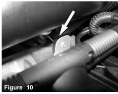
With T30 torx bit, loosen and remove the screw holding in intake tube neer fire-wall on engine.
