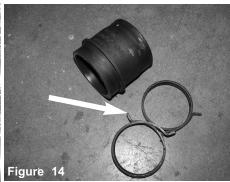
Remove complete stock turbo coupler and clamps shown above.
