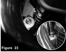
Secure the bracket on intake tube using provided M6 washer and nut. Tighten the nut using 10mm socket and ratchet.
