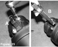
A) With T20 security bit loosen the 2 screws holding. B) Remove MAF sensor.
