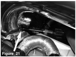
Tighten the remaining clamp on step hose using 8mm nut driver.
