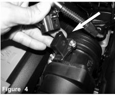
Disconnect MAF sensor harness and set aside.
