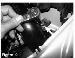
With 10mm socket and extension, loosen the bolt hold- Remove the plastic snorkel assembly. ing in the plastic snorkel assembly.
