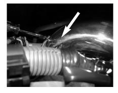
Tighten the clamps on throttle body using 8mm nut
