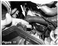
Pull back the ECU harness that is attached to the back of the bottom half of air box.
