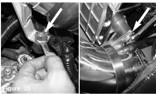
Position for the best possible fit. Make sure nothing is hitting or rubbing. Re-tighten the vibra mounts if necessary for better fit.
