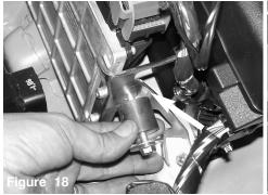
Attach the Vibra mount to the hole on bracket on the ECU. Secure the backside using M6 washer and nut.
