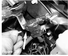
With the provided M5 hex screw, secure to the bracket on tube.
