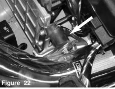
Secure the bracket and tighten using provided M6 nut and washer.
