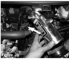
Install the upper intake assembly and position to the throttle body and bracket to the vibra mount.
