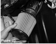
Attach the filter to the intake tube and tighten using 8mm nut driver.
