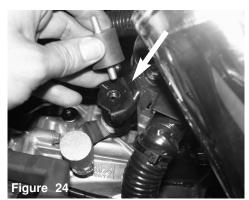
Attach vibra mount to the stock location of air box mounting thredded insert.
