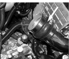
Attach hump hose with clamps provided to the lower intake tube. Do not tighten.
