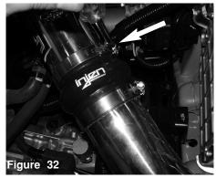
Tighten the clamps on the hump hose using 8mm nut driver.
