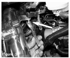
Tighten using 8mm socket with ratchet.
