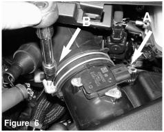
A) Disconnect the MAF sensor harness and harness clips attached to the intake tube. B) Loosen the clamp on air box using 10mm socket or wrench.
