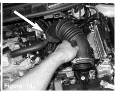
With pliers, pinch the clamp on throttle body and remove the stock intake tube.
