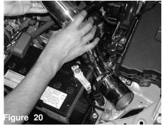
Install the lower intake tube into vehicle between the battery harness, rotate and position the bracket to the vibra mount.
