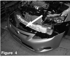
For easier installation, remove the bumper cover to allow for the filter installation of the cold air intake
