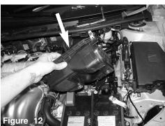
Remove the bottom half of air box out of vehicle.
