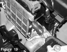
Should look like image above, secure and tighten using 10mm wrench.
