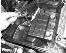
With 10mm socket or wrench, loosen and remove the 3 bolts holding in bottom half of air box.
