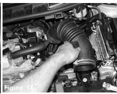
Remove the stock intake tube.
