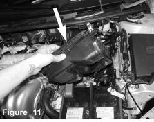
Pull back the ECU harness that is attached to the back Remove the bottom half of air box out of vehicle.
