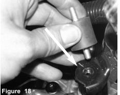
Install the vibra mount to the factory air box mounting location and secure.
