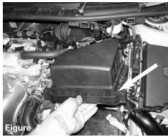
Un-clip the upper half of air box and remove.
