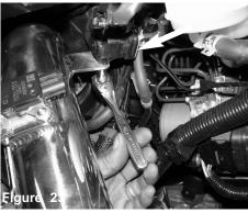
Tighten using 8mm socket with ratchet.
