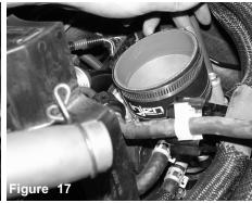
Install the 3" straight hose with clamps to the throttle body.
