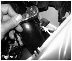
With 10mm socket and extension, loosen the bolt holding in the plastic snorkel assembly.
