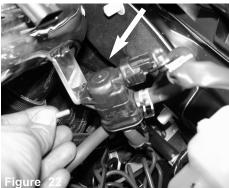
With the provided M5 hex screw, secure the VSV valve to the bracket on tube.
