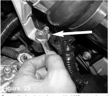
Secure the bracket using provided M6 nut and washer, tighten using 10mm socket or wrench.
