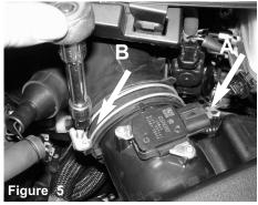
A) Disconnect the MAF sensor harness and harness clips attached to the intake tube. B) Loosen the clamp on air box using 10mm socket or wrench.
