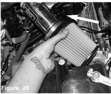
Install the air filter and attach to the intake tube and tighten using 8mm nut driver.
