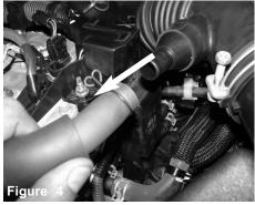
Pull back the crank case line from stock intake tube.
