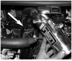
Install the intake tube and position to the throttle body and bracket to the vibra mount.
