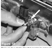
There are four plastic clips that need to be removed from the mud flap. There are three clips to the outside and one clip to the inside of the mud guard.
