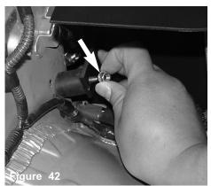
The ascending line is reconnected to the motor pump again.
