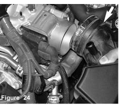
Once you have loosened the clamp, continue to pull the air intake duct from the throttle body.
