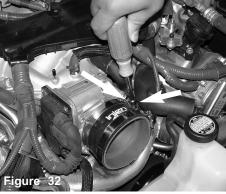
Once the grommet is aligned, continue to press it into the pre-drilled hole in the reservoir bottle.
