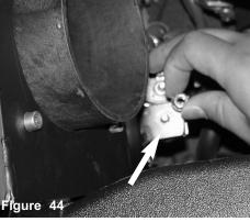
The extended wire harness is lined up to the motor pump.
