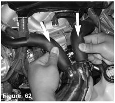
The mass air flow sensor is now inserted into the sensor adapter as shown above.
