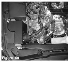
The vacuum hard pipe is pulled out of the engine compartment.
