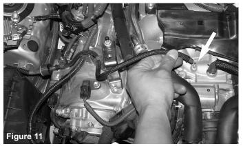
The vacuum line with the one-way check valve is pulled from the vacuum port.
