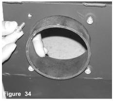
The motor pump is aligned and pressed into the grommet as shown above.
