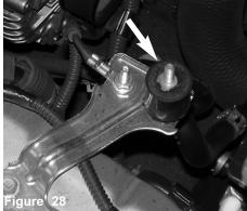
The m6 bolts are fastened with an allen as shown above.
