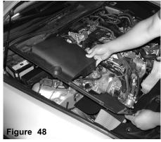
The stand-off is firmly pressed into the grommet
