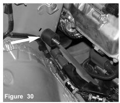
The top bracket m6 bolts are now fastened to the reservoir bottle.
