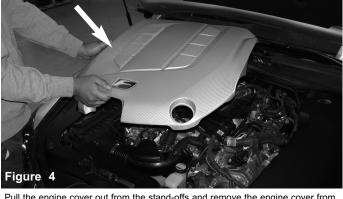
Pull the engine cover out from the stand-offs and remove the engine cover from the engine compartment.
