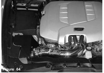
Periodically, check the fitment of both intake systems. Normal driving conditions may loosen nuts, bolts and clamps causing intakes to shift resulting in damage to other automotive parts.
