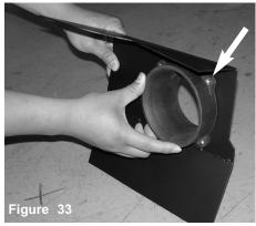
The reservoir motor pump is pressed into the grommet as shown above.
