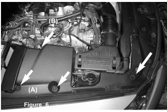
Plastic Clips shown in Figure (A) will be removed and nut shown in figure (B) is also removed.
