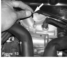
The 3mm vacuum cap is pressed over the vacuum
