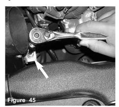
The harness clip is now re-connected to the motor pump.
