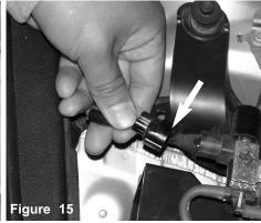
The harness clip is also removed from the vacuum switching valve.
