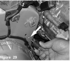
The top, strut tower mount bracket is aligned to the reservoir bottle, two m6 x 10mm bolts are used to secure bracket in place.
