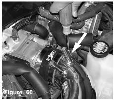
The clamp on the throttle body side is tightened at this point.
