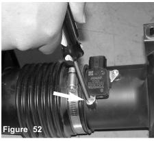
Loosen and remove the two screws holding the mass air flow sensor in the sensor housing.
