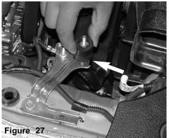
The side fender well bracket is aligned to the press nuts located on the side of the reservoir bottle. Use two m6 x 10mm hex bolt to secure the bracket.
