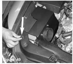
The vacuum hard pipe is pulled off the crankcase port.
