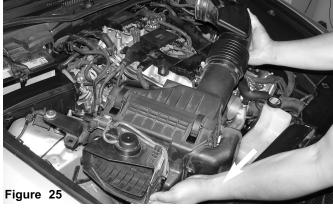
The air box cleaner is now ready to be moved from the engine compartment.
