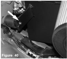
Take the m6 x 10mm bolt and and screw it into the pre-tapped fender well hole.
