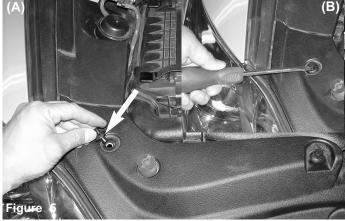
Remove the plastic clip on the passenger side of the front shroud (A) Pop center pin, lift (B)and remove clip as shown above.
