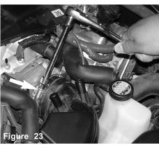
Loosen the throttle body clamp over the air intake duct.
