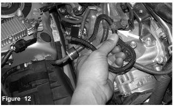
The reinforced vacuum hose is detached from the metal clip as shown above.
