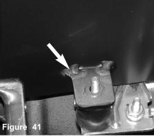
The side bracket is now tightened using an allen.
