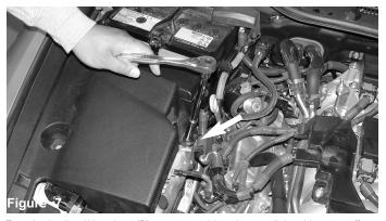
Two plastic clips (A) and nut (B) are removed in order to pull the side cover off.
