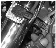
Use the stock screws to secure the MAFS in the sensor adapter (A). Firmly press the electrical sensor connector into the MAFS until it clicks in place (B).
