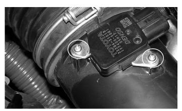
Loosen and remove the two sheet screws that fasten the MAFS to the sensor housing.
