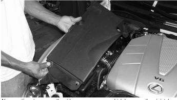
Now, continue to remove the side accessory cover which lays over the air intake box cleaner.
