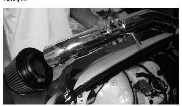
Slip the three inch filter over the end of the intake until it butts up against the filter stops. Once the filter has been firmly placed, continue to tighten the filter neck clamp.
