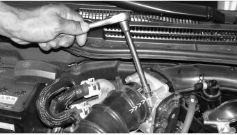
Loosen the only remaining metal clamp which secures the air duct to the throttle body as shown above.
