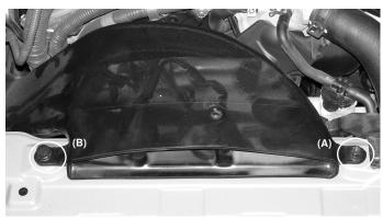
Loosen and remove one bolt (A) depress and pull the last remaining plastic clip (B) now holding the air scoop in place.
