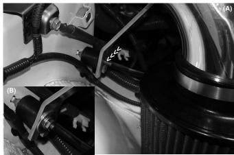
The intake bracket is aligned to the vibra-mount stud (A). Use the m6 flange nut and fender washer to secure the intake in place (B).
