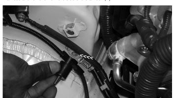
Once the screw has been removed, continue to place the vibra-mount into the pre-tapped hole as shown above.
