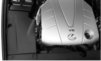
Once the intake has been fitted for a perfect fit, continue to replace the plastic air intake scoop, passenger side accessory cover and the engine cover.
