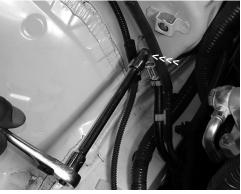
Use a 10mm socket and ratchet to remove the screw that secures the grounding wire to the fender well.
