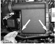
On front of the factory airbox cleaner, unclip the front two retaining clips
