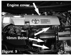
Lift up on the engine cover and remove temperarely and then remove three 10mm bolts attached to the lower air box cleaner
