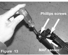
Use a phillips screw driver and remove the two screws attaching the MAF sensor to the upper airbox cover.
