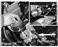
Figure A: Place the 2.5" straight hose and two .040 clamps onto the throttlebody. Figure B: Use a 8mm nut driver to tighten the throttlebody clamp for now.
