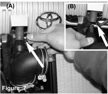
Figure A: Press on the pressure clamp on the air duct breather port. Figure B: Disconnect the breather line from breather duct on the air duct tube.
