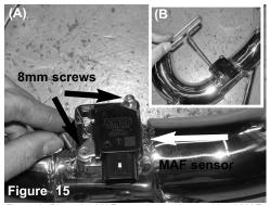
Figure A: Place the MAF sensor onto the machined MAF sensor pad on the Injen intake pipe and use two M4x10 button head screws to secure it. Figure B: Use a 2.5mm allen driver and tighten the two 4mm screws
