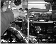
Place the factory breather line to the long 5/8 nipple welded to the pipe.
