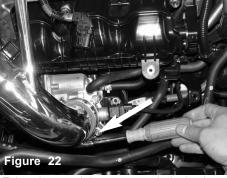
Tighten the second clamp tp secure the intake pipe on the 2.5" hose that was already on the throttlebody
