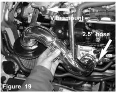
Lower the intake tube into the engine bay and push the non-filter end of the tube into the 2.50" straight hose. Then align the mounting bracket onto the vibramount
