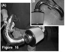
Figure A: Place the 2.5" filter onto the pipe end with the tighter radius. Figure B: Pipe shown with the filkter on the correct end.
