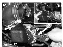
FigureA: Use a set of niddle nose pliers and losen the pressure clamp on the throttlebody air duct. Figure B: Now remove the thottlebody air duct.
