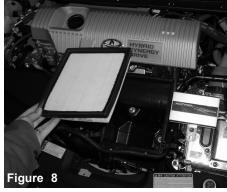
Remove the air filter panel to access the two 10mm bolst attaching the lower airbox cleaner to the engine.
