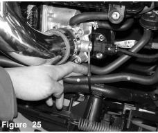
Zip tie the loose coolant line that was originally attached to the factory airbox.
