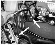
Remove the last two 10 mm bolts attached to the lower airbox cleaner.
