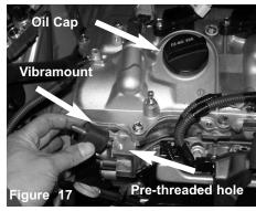
Place the M8 vibramount onto the pre-threaded hole next to the valve cover. Use the oil cap in the photo to reference the location of the pre-threaded hole
