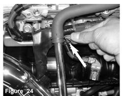
Press the pressure clamp back onto the factory breather line.
