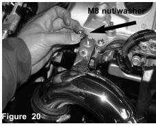
Place a M8 nut and washer onto the vibramount
