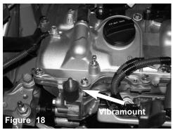
Vibramount mounted to cylinder head
