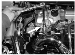
Once the intake tube is adjusted for best fitment, use a 13mm socket and 3/8 rachet and tighten the M8 bolt securing it to the bracket on the pipe
