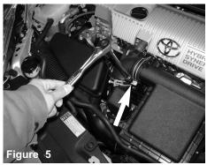
Loosen clamp from throttlebody air duct to air box cleaner using a 10mm socket and 3/8 rachet
