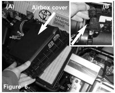
Figure A: Lift up on the airbox cover. Figure B: Disconnect the MAF sensor harness from the MAF sensor on the airbox cleaner.
