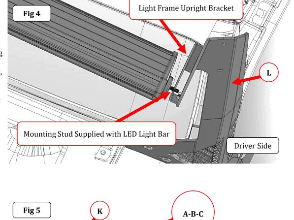
**Step-4** Attach a retainer plate to the light bar mounting stud using the fasteners included with the light bar, and attach the opposite end of the retainer plate to the light frame upright using (1)  $\frac{1}{4}$ " x  $\frac{3}{4}$ " button head screw, (1)  $\frac{1}{4}$ " lock washer and (1)  $\frac{1}{4}$ " flat washer, (Fig 5). Repeat for the passenger side.
