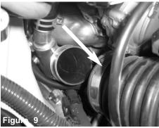
With 8mm nut driver or flat headscrewdriver, loosen the clamp holding in the stock intake tube on the turbo and remove.
