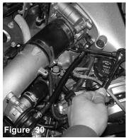
Installation of the upper intercooler pipes, Note: installation is the same for both sides, photos are of passenger side only.
