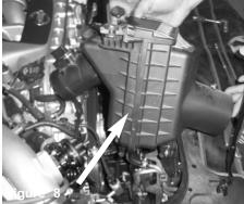
Carefully lift and pull out the air box.
