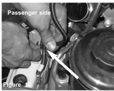
Pull back the engine ground fitting from the bracket located on the passenger side frame of vehicle. This will allow for the installation for the vibra mount.
