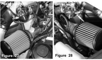
Align the intakes for best possible fit. Once you have aligned and made sure that the length of the intakes are free from any moving parts, continue to tighten all nuts, bolts and clamps.
