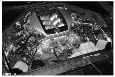
Congratulations! You have just completed the installation of the best cold air intake consisting of the patented MR Technology and now patent pending Air Fusion. Periodically, check the fitment of the intake for possible shifting that may occur over time or driving conditions.
