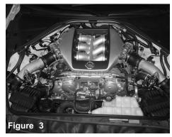
Complete stock intake system, Disconnect battery. Remove both sides of stock intakes. Passenger side shown, both are exaxtly the same when removing.
