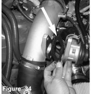
Loosen the 2 bolts holding in the blow off valve using  $\overline{12}$ mm socket or wrench, pull back and save the factory gasket.
