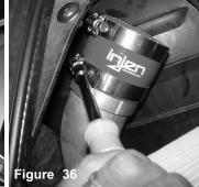
Now carefully pull back the sensor harness line, and remove the factory upper intercooler pipe. Install the 2-3/8" hose to the factory intercooler pipe.
