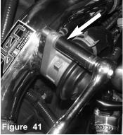
Re-install the blow off valve to the new intercooler pipes. Re-use the factory gasket and bolts. Secure and tighten using 12mm socket and ratchet.
