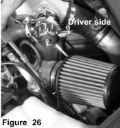
Install filters and secure using 8mm nut driver. Tighten all remaining clamps.
