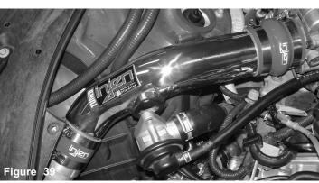
Position for the best possible fit and tighten all the clamps on the intercooler pipes.
