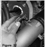
Loosen the screw holding in the temperature sensor, save screw for later install. Pull out the temperature sensor.
