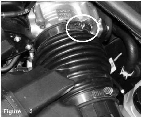
Figure 3 use an 8mm nut driver or screwdriver to loosen the throttle body clamp.
