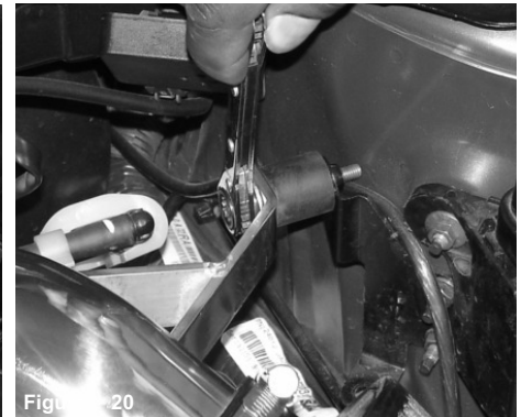
Figure 20 Manual and auto transmission: Use a 10mm wrench and secure the 10mm nut to the intake bracket
