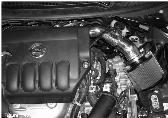
Figure 43 Periodically, check the fitment of the intake and heat shield. Normal wear and tear may cause shifting of the intake that may cause damage to the intake. Failure to perform monthly preventative maintenance will void the warranty of this intake system.
