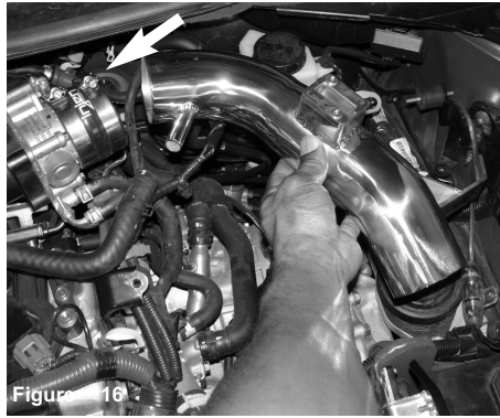
Figure 16 Lower the air intake pipe into the engine compartment and press the smaller end of the pipe into the throttle body hose.
