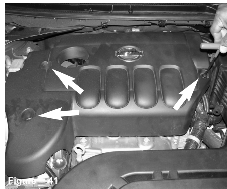
Figure 41 The three stock m6 bolts are used to fasten the engine cover again.
