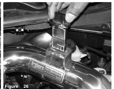
Figure 26 Insert the original mass air flow sensor into the machined billet sensor adapter.
