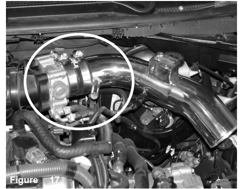
Figure 17 The intake is now attached to the throttle body.
