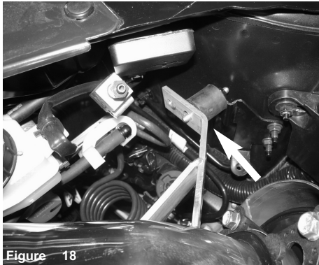
Figure 18 Manual and auto transmission: Align the 3/8" hole on the intake bracket to the vibra mount from figure 15.
