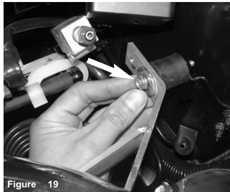
Figure 19 Manual and auto transmission: The m6 flange nut and fender washer is used to fasten the air intake to the vibra-mount stud.
