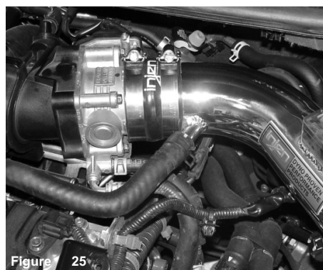
Figure 25 Once the crankcase vent hose has been pressed into the intake port, continue to re-use the tension clamp to secure the hose in place.
