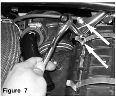
The two bolts on the boost solenoid bracket are loosened and removed from the air box.
