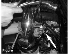
Using the factory nut, tighten the boost solenoid using 10mm socket with ratchet.
