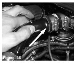
Install the hard line into the hose, and position for the best fit.
