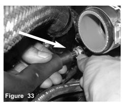
Re-install the crank case line to the fitting on intake tube and secure using the factory clamp using pliers.
