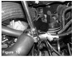
Loosen clamp on hard line for a light rotation.
