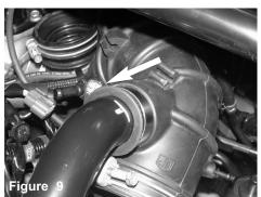
The blow off return line clamp is loosened prior to removing the air box. The hard line is removed from the intake tube.
