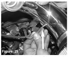
Now attach the vacuum line to the fitting on the intake tube and secure.
