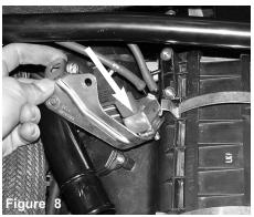
The bracket is pulled off the air box cleaner top.
