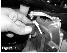
Install the male/female vibra mount to the ECU bracket
