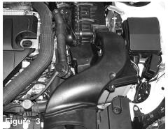
Stock engine compartment. Disconnect the MAF sensor and battery before the installation.
