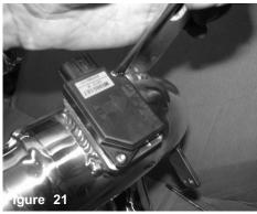
Secure the MAF sensor using the provided M4 screws. Tighten using 2.5mm allen key.
