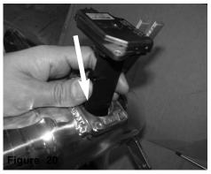
Install the MAF sensor into the new intake tube
