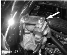
Attach the boost solenoid to the bracket on the intake tube. There is another hole cut out for the notch on the booster solenod for it to sit flush on bracket.
