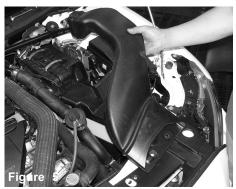
Once you have removed the two plastic clips, continue to remove the front air scoop.
