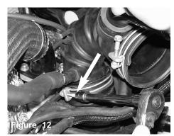
The air duct clamp is loosened connected on the turbo inlet.
