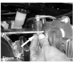
Position the bracket to the vibra mount and secure using the M6 nut and washer. Do not tighten.
