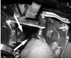
Position the intake tube for the best possible fit. Tighten the vibra mount using 10mm socket and ratchet.
