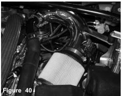
Align the intakes for best possible fit. Once you have aligned and made sure that the length of the intakes are free from any moving parts, continue to tighten all nuts, bolts and clamps. The upper intercooling pipes, SES1837ICP is now sold separately.
