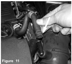
Once the tension clamp as been pulled back, pull the crankcase vacuum hose from the air duct port.
