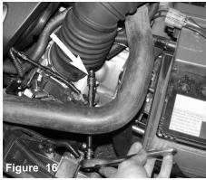
The air duct clamp is now loosened from the throttle body.
