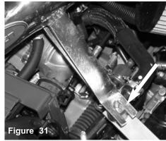
As the intake is inserted into the throttle body hose the intake bracket is aligned to the vibra-mount stud.
