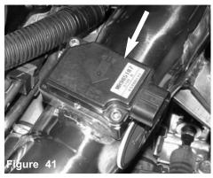
The mass air flow sensor is now installed in the machined sensor adapter.
