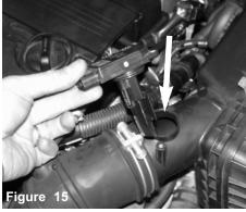
The mass air flow sensor is now pulled out of the sensor housing.
