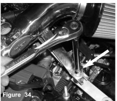
The fitment is checked again prior to tightening the m6 flange nut on the intake bracket and vibra-mount.
