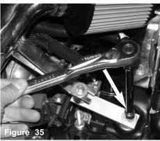
The m6 nut is now tightened over the extension brack-
