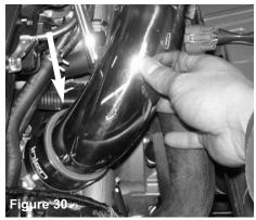
The lower end of the intake is inserted into the throttle body hose.
