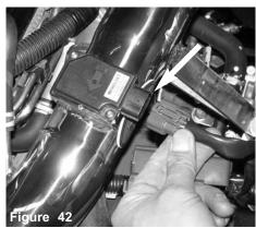
The harness clip is pressed over the mass air flow sensor until it snaps in place. You are now ready to re-install the front air scoop back to its original location.
