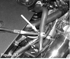
Use the needle nose pliers o compress the tension clamp to slip over the vacuum hose.
