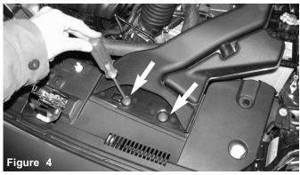
A phillips screw driver is used to loosen the two plastic clips.
