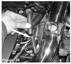
The crankcase vacuum hose is now pressed over the intake vacuum port.
