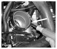
Once you have positioned the hose in place, continue to tighten the hose clamp located over the throttle body.
