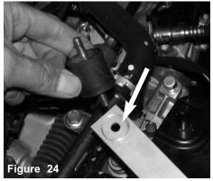
The vibra-mount is aligned to the end of the extension bracket and inserted into the hole.
