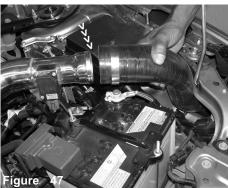
Once you have lower the lower end into the resonator opening, continue to align the intake to the primary aluminum intake.
