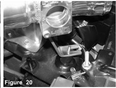
The intake bracket is sitting flush over the vibramount stud.
