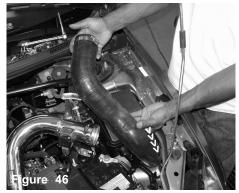
The secondary silicone hose is now lowered into the engine compartment.
