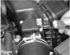
Depress the plastic tab and pull the electrical sensor harness from the mass air flow sensor.
