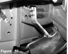
Use the m6 flange nut and fender washer to fasten the intake bracket to the vibra-mount stud.
