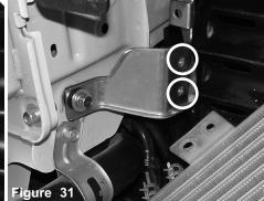
The two m8 bolts fastened to the zinc plated brace have been loosened and removed. The oil cooler is now detached from the brace.
