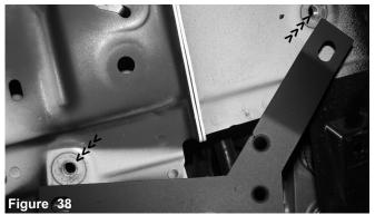
The new oil cooler bracket is aligned to the car frame with the press nuts facing inward towards the car frame.
