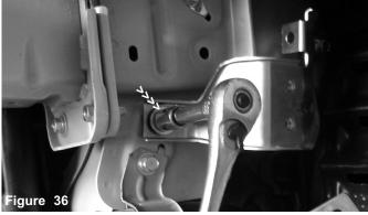
The last m8 bolt is loosened and removed from the zinc plated brace. Once the m8 bolts have been removed , continue to remove the brace.
