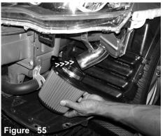
Align and press the filter neck over the intake end.
