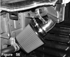
Once the intake end has butted up against the filter stops, continue to tighten the filter neck clamp.
