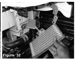
Once all three bolts have been removed, continue to remove the oil cooler from the two braces.
