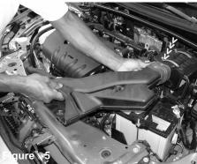
Pull the front scoop from the air box cleaner and remove it from the engine compartment.
