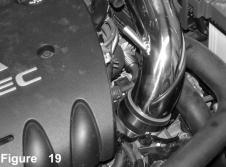
Once the intake has been pressed into the throttle body hose, continue to align the intake bracket to the primary vibra-mount stud.
