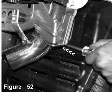
Tighten the hose clamp on the extended intake shown above.
