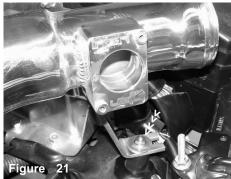
The m6 flange nut and fender washer are used to fasten the intake bracket to the vibra-mount stud.
