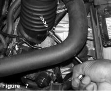
Loosen the air duct clamp from the throttle body hose.
