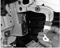
The L-shape zinc plated brace is now removed from the top frame.
