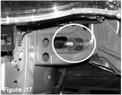
The secondary vibra-mount is now sitting flush along the bumper area along the frame.
