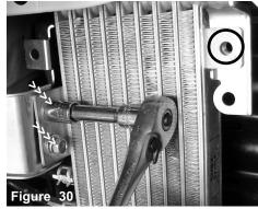
Once you have removed the top bolt as shown above circled, continue to remove the two additional m8 bolts fastened to the zinc plated brace.
