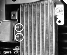
Applicable to all GTS models: Oil cooler that will be relocated in order to make room for the filter.
