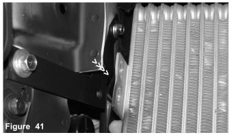
The oil cooler is now aligned to the new bracket as shown above.
