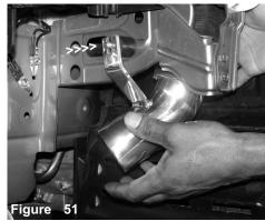
Press the extended intake to the secondary silicone hose and align the intake bracket to the vibra-mount stud.
