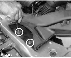
Unscrew both bolts and pop the plastic clip out of the front air scoop.
