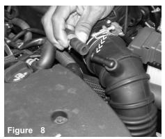
Remove the crack case breather hose from the air intake port.
