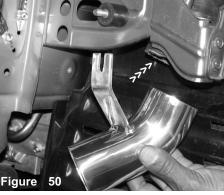
Align the extended intake to the secondary silicone hose as shown above.
