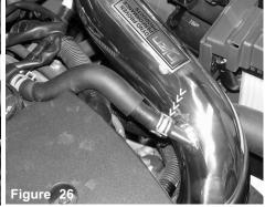
Once you have pressed the breather hose over the intake air port, continue to use the tension clamp over the breather hose. All non-GTS models, proceed and go to figure 46 to continue.
