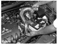
The primary intake is now lowered into the engine compartment and pressed into the throttle body hose.
