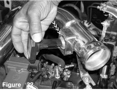
The mass air flow sensor is now inserted into the sensor adapter. A dab of light oil is used on the O-ring to prevent kinking or tearing of the O-ring.
