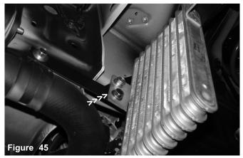
Both m8 x 16mm bolts are now installed and holding the oil cooler in place.
