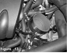
Press the 2 3/4" straight hose over the throttle body. Slip two power-bands over the 2 3/4" hose and tighten the clamp over the throttle body.
