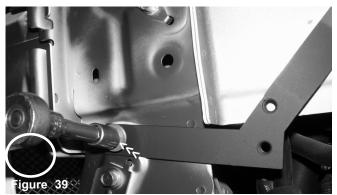
The first m8 x 21mm bolt is aligned to the frame to  $% \left( f_{x}^{2}\right) =0$  fastened the new bracket.
