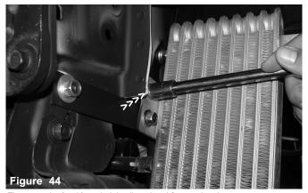
The second m8 x 16mm bolt is aligned and fastened to the upper press nut.
