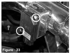
Use the m4 bolts provided in this kit to fasten the mass air flow sensor to the sensor adapter.
