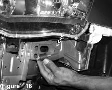
The secondary m8 vibra-mount is now aligned to the frame in the bumper area.
