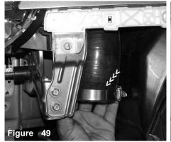
Slip one power-band over the end of the secondary silicone.
