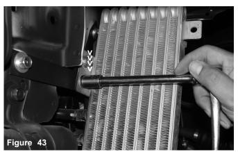
The first m8 x 16mm bolt is aligned and semi-tightened to the lower press nut.
