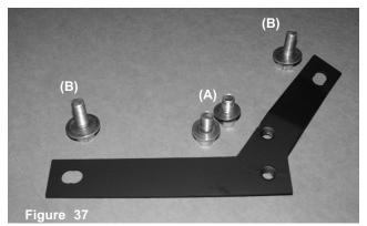
The stock m8 bolts are now used with the new oil cooler bracket. The two m8 x 16mm bolts (A) are fastened to the press nuts while the two m8 x 21mm bolts (B) are used to attach the entire bracket to the car frame.
