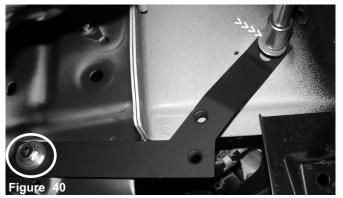
Once the first m8 bolt is semi-tightened as circled above, continue to align the second m8 x 21mm bolt to the car frame.
