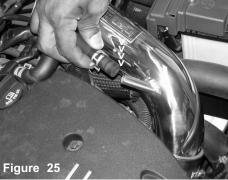
The stock crank case breather hose is now aligned to the intake port as shown above.
