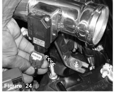
Press the electrical sensor harness clip over the mass air flow sensor until you hear them snap together.
