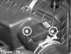
Unscrew the two m4 bolts from the mass air flow sensor housing. This will allow you to remove the mass air flow sensor from the sensor housing.
