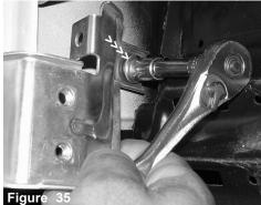
The final two m8 bolts are removed from the larger zinc plated brace that is attached to the car frame.
