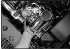
**23.** Install the lower intake tube assembly. Position the tube to upper intake tube and bracket to the vibramount.
