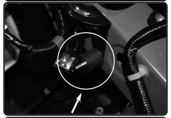
**22.** Now secure the bracket using provided M6 Vibramount
