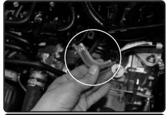
**10.** Remove the bracket from the vehicle. Save screw for later install.
