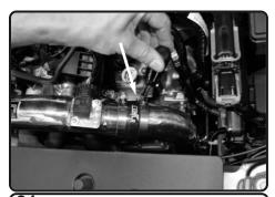
**24.** Attach the 2 intake tubes together, and tighten clamps. *Note:re-adjust if necessary.*
