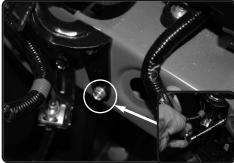
**21.** Locate the air box bracket on the vehicle frame, loosen the 10mm hex screw and remove using 10mm socket or wrench.
