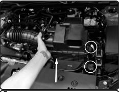
**5.** Loosen the 2 bolts holding in the air box and remove. Lift up and remove the complete stock air box assembly out of vehicle.
