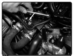
**12.** Now install the new provided bracket to the engine, secure using the original screw. Tighten using 10mm socket or wrench.
