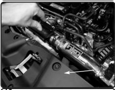
**18.** Tighten the clamp on straight hose.
