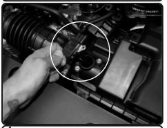
**4.** Remove the sensor from the air box. Save screws for later install.
