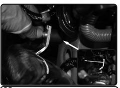
**25.** Secure the bracket using provided nut and fender washer. *Adjust intake for proper clearance and fitment.* Secure and tighten the vibramount.
