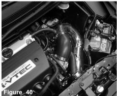
Your intake installation is now complete. Reinstall the battery and all of its components in the reverse order of removal and go over all your clamps and fitting to make sure they are snug. Check the clearance on the components in the engine bay. Start the car and make so will void the warranty. sure there is no CEL or coolant leaks. Go through all the gears and make sure they engage properly. You may now take the vehicle for a test drive.
