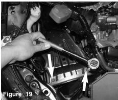
Use a 12mm socket and rachet and remove the two 12mm bolts on the battery support bracket attached to
