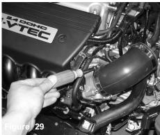
Now tighten only the clamp on the throttlebody side.
