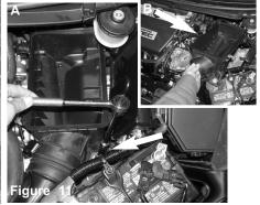
Figure A: Use a 10mm socket and rachet to remove the bolt on the front right side of the lower air box assembly. Figure B: Lift up on the back side of the lower air box assembly to detach the rear grommets and then pull the lower box assembly out.
