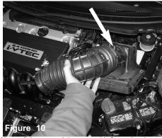
Now pull the upper air box assembly forward and out.
