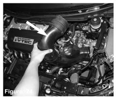
Pull firmly on the lower resonator duct to detach it from the resonator box located in the front bumper. This air duct will no longer be used.
