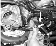
Place the supplied 1/4" plastic coupler onto the throttlebody coolant line.
