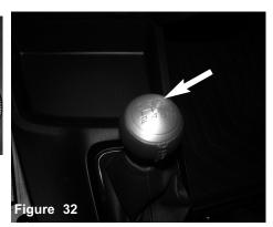
Place the car into 5th gear. The shifter counter weight lever in the engine bay is in its highest position when in 5th gear and you will have to check for pipe clearance later in figure 37
