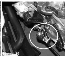
Vibramount shown mounted to the clutch slave cylinder fluid line bracket
