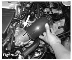
Place two clamps and the 60 degree 2 7/8X3.00 elbow with the 2 7/8" end onto the throttle body
