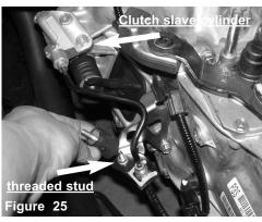
Locate the threaded stud on the clutch slave cylinder line bracket and screw the female side of the supplied male/female vibramount onto it.
