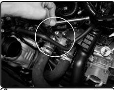
**6.** Locate the bracket on the engine holding in line. Pull back harness and loosen the bracket using 10mm socket or wrench.
