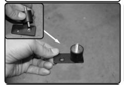
**8.** Now install the M6 vibramount to the thredded fitting on the provided bracket. Secure and tighten.
