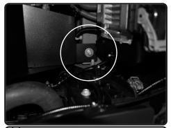
**14.** Secure the bottom of the heatshield to the thredded insert on vehicle frame using provided M6 screw with fender washer.
