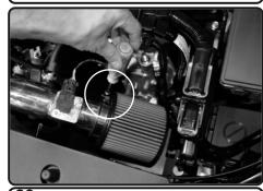
**23.** Install the filter and tighten clamp using 8mm nut driver.
