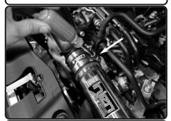
**20.** Secure and tighten the clamp on turbo housing.
