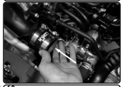
**10.** Install the 2-3/8" straight hose with clamps to the turbo housing. Tighten the clamp on the housing only.
