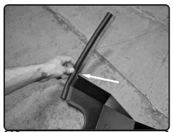
**12.** Now install the rubber trim to the heat-shield. Cut a notch in corner for easier installation.
