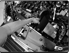
**13.** Install the heatshield into the vehicle and position.
