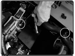
**16.** Secure and tighten both screws using 10m socket or wrench on heatshield.
