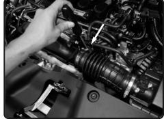
**7.** Loosen the clamp on the turbo housing using phillips screwdriver.
