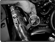
**18.** Secure the vibramount using provided M6 nut and fender washer, tighten using 10mm socket and fender washer.
