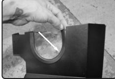
11. Install the vinyl trim to the hole cut out on heatshield.
