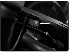
**15.** Secure the tab to the front of the raiator support. Locate the thredded insert and secure using provided M6 screw and fender washer.
