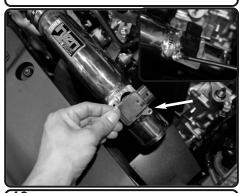
**19.** Install the MAF sensor into the intake tube. Secure using factory screws and tighten.
