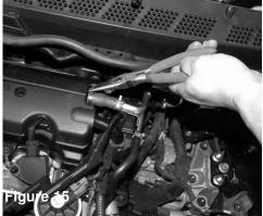
Use a plier and loosen the pressure clamp from the CCV line connected to the valve cover.
