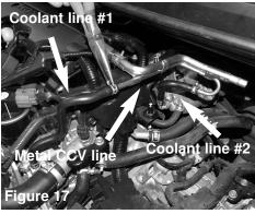
There are two coolant lines attached to the metal CCV line. Coolant line 1&2 will be disconnected from the metal CCV line and reattached together using a 1/4" plastic coupler later in figure 20
