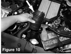
Firmly pull the rubber air duct off the front of the lower air box assembly.
