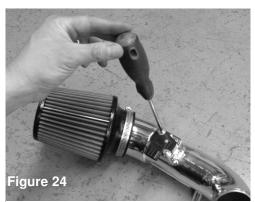
USe a phillips screw driver and tighten the two screws to secure the MAF sensor to the machined MAF sensor pad.
