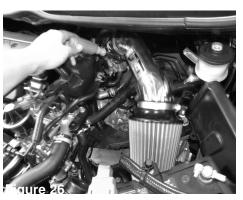
Due to the short legth of the intake pipe, it does not require a mounting bracket. Position the intake for best fitment and then tighten the clamp to secure pipe to the throttle body.
