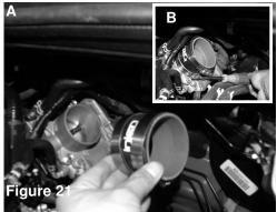
Figure A: Place the 2.5" straight hose with 2 #40 clamps onto the throttle body. Figure B: Use a 8mm nut driver and tighten the clamp on the throttle body only for now
