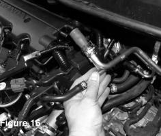
Detach the metal CCV line from the valve cover.
