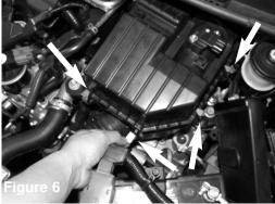
Release the four metal tabs attaching the lower and upper air box assemblies.
