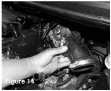
Remove the rubber throttle body air duct to air lower air box assembly out
