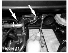
Use a 5.5mm socket and rachet and loosen the clamp onthe lower air box assembly air duct to throttle body. Then continue to loosen the clamp on the throttle body side.
