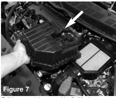
Pull the upper air box assembly off of the lower assembly
