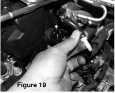
Attach the supplied 1/4" plastic coupler to one end of the coolant line.
