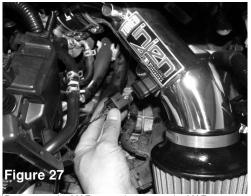
Re-connect the MAF sensor harness to the MAF sensor on the intake pipe.
