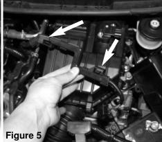
Press on the release tabs on the MAF sensor harness plastic channel to remove the harness from the air box assembly.
