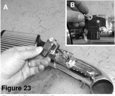
Figure A: Place the MAF sensor into the welded machined MAF sensor adapter. Figure B: Re-use the factory MAF sensor screws to attach MAF sensor.
