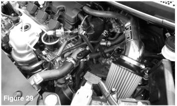
Check the alignment and fitment of the entire Injen intake. Once you have check for possible air leaks, rubbing or rattling, continue to tighten all nuts, bolts and clamps.
