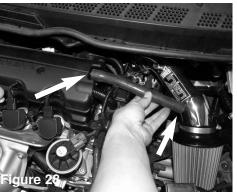
Connect one end of the 15mm vacuum line to the breather line on the valve cover and the other end to the welded nipple on the intake pipe.
