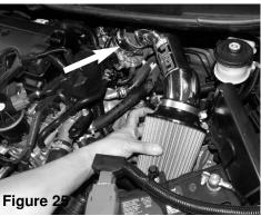
Position the intake pipe into the engine bay and place the end of the intake pipe into the throttle body
