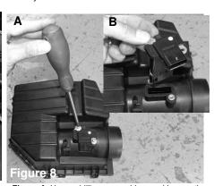
Figure A: Use a phillips screw driver and loosen the two screws on the MAF sensor. Figure B: Pull the MAF sensor out of the air box housing. This sensor will be reused in this intake kit.
