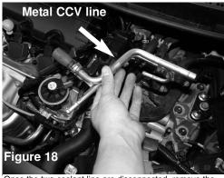
Once the two coolant line are disconnected, remove the metal CCV line. This metal CCV line will no longer be used in this intake kit.
