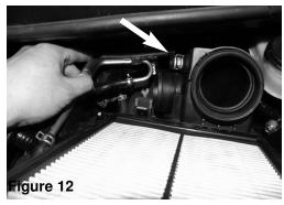
Pull the metal CCV / coolant line out of the lower air box assembly
