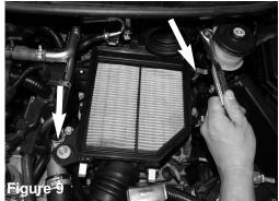
Use a 10mm socket and rachet and loosen the two 10mm bolts connecting the lower air box assembly to the engine.
