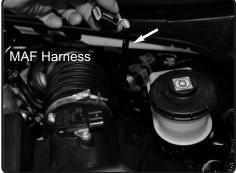
7. Disconnect the MAF sensor harness. Pull back the line away from the air box.
