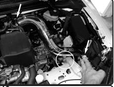
**18.** Now install the intake into vehicle. Position the tube to the throttle body and the bracket to the vibramount.
