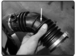
**4.** Now Lift up and remove the stock intake tube out of the vehicle.
