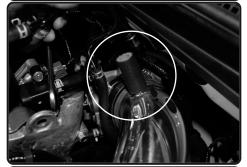
**22.** Now install the 12mm hose to the fitting on intake tube.
