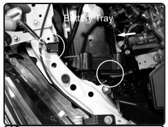
**12.** Loosen the 2 screws holding in the ECU bracket. Remove battery tray.
