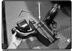
**10.** Now pull down and remove the air box resonator out of vehicle.
