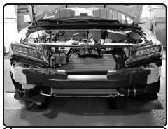
1. Stock intake system shown. Remove the front bumper cover.
