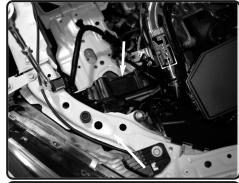
**19.** RE-install the ECU and secure. Adjust tube and tighten clamp on throttle body using 8mm nut driver.
