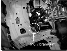
**15.** Install the M6 vibramount to the threaded fitting from stock air box. Secure and tighten.
