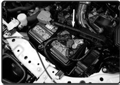
**21.** Re-connect and secure the battery assembly. Verify the intake tube has all the clearance.
