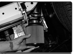
**25.** Install the air filter to the intake tube. SEcure and tighten using 8mm nut driver.
