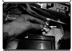
**20.** Secure the bracket using provided M6 nut and fender washer and tighten using 10mm socket or wrench.
