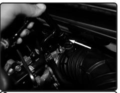
**2.** Carefully lift up and remove the crankcase line out of the intake tube.
