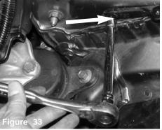
Use a 10mm socket and 3/8 ratchet to remove the lower 10mm bolt attaching the support bracket on the driver side shock tower.
