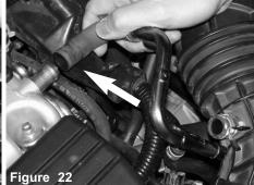
Then remove the PCV breather from the valve cover. Disconnect the air box duct from the throttle body.
