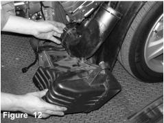
Firmly pull down and out to remove air resonator box. This may require some aggressive pulling when removing the resonator box.
