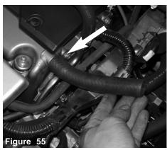
The 15mm hose is pressed over the crankcase vacuum port.
