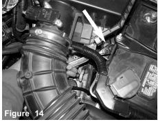
Proceed to remove the second 10mm bolt as shown above. Do not remove the air box just yet.
