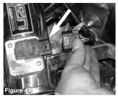
The electrical harness clip is now pressed over the mass air flow sensor. Press firmly until it snaps in place. Page 5 of Part# SP1432
