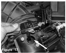
Carefully, pull the air mass sensor from the factory air box, this will also be use later.
