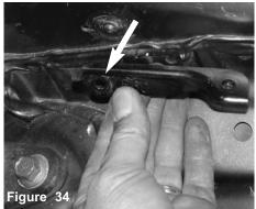
Remove the 10mm bolt and support bracket, this is where the vibra-mount will be installed.
