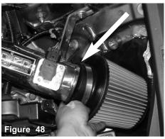
**On rainy days**, the primary intake can be used as a short ram, simply press the filter over the end of the intake and tighten the filter clamp.
