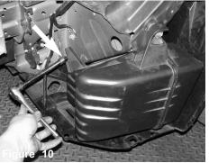
With the front bumper removed, you can now access the air resonator box located on the driver side. Use a 10mm 3/8 socket and ratchet to remove the first 10mm bolt.
