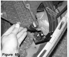
Now reattach the harness to the fog light on the the bumper of the car.
