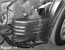
Remove the second 10mm bolt. Now the air resonator box is ready for removal.
