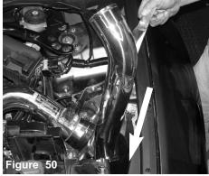
The secondary intake is lowered into the resonator opening and aligned to the primary intake.
