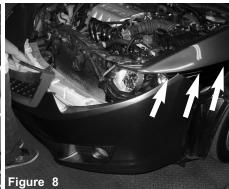
Firmly pull the sides of the front bumper outwards until the bumper unlatches from the clips located below the headlights.
