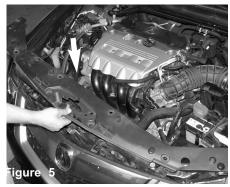
Once all plastic plugs have been removed, continue to pull the top shroud out of the engine compartment.
