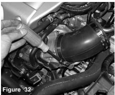
Once the step hose is placed onto the throttle body, you can tighten the clamp on the throttle body Side. Leave the remaining 048 clamp loose for now.
