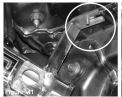
Line the primary intake bracket to the vibra mount stud located on the shock tower mount.
