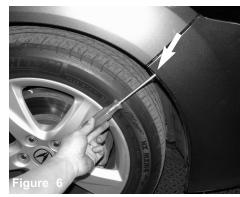
Remove one phillips screw on each side of the front bumper using a phillips screw driver
