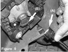
Passenger side bumper- Pressing down on the harness center tab (A) , unclip the foglight harness from the bulb base (B) Repeat step for the driver side fog lamp.
