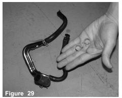
PCV hard pipe removed from the engine compartment. The hose spring clamps are the only items reused to hold the coolant line in place.
