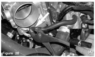
Retain the spring clamp on the end of the coolant(A) Press the thermoastate coolant hose over the throttle body coolant inlet (B).
