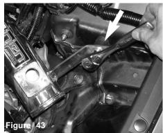
Use a 10mm 3/8 socket and ratchet to tighten the M6 nut to the vibra mount.
