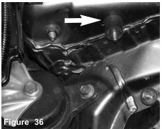
The vibra-mount is screwed in until it sits flush with the strut tower mount.
