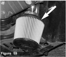
Once the intake end is sitting flush to the filter stops, continue the tighten the filter neck clamp.
