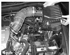
The entire air box and air duct can now pulled out of the engine compartment
