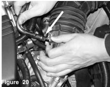
Pull the steel PCV breather tube out of the factory air box duct.
