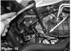
Use a 10mm 3/8 socket and ratchet to loosen clamp on the factory air duct connected to the throttle body.
