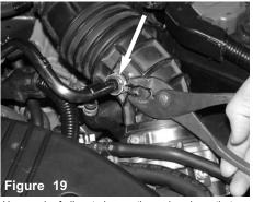
Use a pair of pliers to loosen the spring clamp that secures the PCV breather tube as shown.
