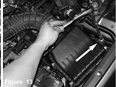
The upper air box is secured with two 10mm bolts. Remove the first one as shown above.
