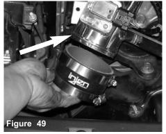
Continuing with the installation of the cold air intake-The 3 1/8" hose is pressed over the end of the intake, use a 8mm nut driver to tighten the clamp over the intake end.
