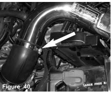
Press the tube with the air mass sensor side into the 2 7/8" X 3 1/4" step hose.
