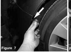
Picture shows removing phillips screw from bumper
