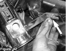
Use one fender washer (X-6010) and one M6 nut (X-6002) to secure the bracket to the vibra mount.
