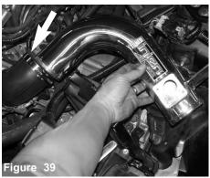
Place the primary tube (longer tube) into the wheel well opening. Make sure the air mass sensor adapter side is on the top side.
