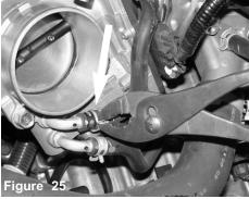
IMPORTANT !!! Make sure the vehicle has cooled down before doing these next steps. Remove the spring clamp from the coolant line just under the throttle body as shown.
