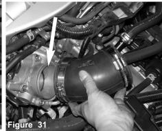
Place one .048 clamp over the hose connected to the throttle body and one clamp over the end of the step hose. Now align the molded hose over the throttle body.
