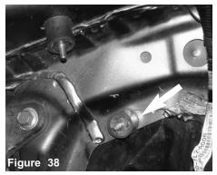
Proceed to screw the Vibra mount in place as shown above. Both vibra-mounts are now installed.
