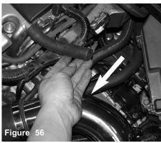
The remaining end of the 15mm hose is pressed over the intake port.
