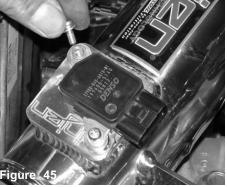
Reuse the two screws that secured the air mass sensor to the factory air box.
