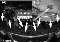
Remove front bumper. Gently pop plastic clips up using a flat head screw driver as shown above (B). There are 7 plastic clips on top and 10 plastic clips on the bottom of the bumper (A).
