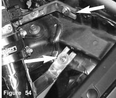
Tighten the m6 flanged nuts to secure the intake brackets to the vibra mounts.
