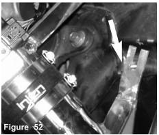
As the secondary intake is pressed into the 3" hose, the intake bracket is aligned to the vibra-mount stud.
