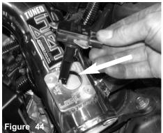
Insert the factory air mass sensor in the the billet adapter as shown.
