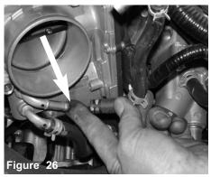
Proceed to remove the coolant line as shown. A little coolant may spill out, which can just be wiped up with a shop rag.
