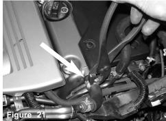
Again with the pliers, loosen the spring clamp that secures the PCV breather to the valve cover.
