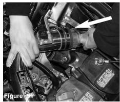
The secondary intake is now pressed into the 3" hose located on the primary intake.
