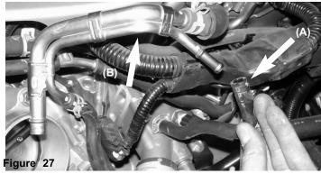
Using pliers loosen the spring clamp on the end of the thermostate hose and pull the hose off the PCV hard-pipe (A) The entire PCV hard pipe is now ready to be pulled out of the engine compartment (B).
