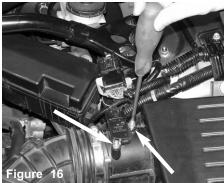
Using a phillips screw driver, unscrew two phillips screws from the air mass sensor. Place these phillips screws to one side because you will be reusing these later.
