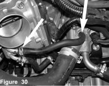
The stock coolant hose is reused and connected directly over the throttle body coolant inlet.
