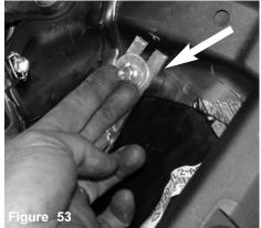
The remaining fender washer and m6 flange nut are used to secure the secondary intake.
