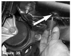
The vibra-mount is aligned to the pre-tapped hole as shown above.
