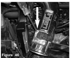
Tighten the two screws securing the air mass sensor the the billet adapter.
