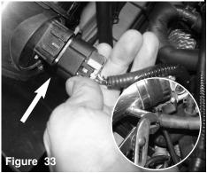
Re-connect the MAF sensor harness. With pliers, secure the crank case line to fitting on intake tube.
