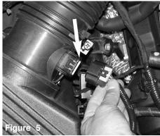
depress the tab on the electrical harness and gently pull on the harness clip.
