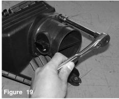
The two bolts are loosened and removed from the mass air flow sensor attached to the air box cleaner.
