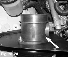
The MAF sensor needs to be positioned like above image or you can damage the sensor. See step 29.
