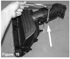
The clamp over the air duct is loosened and the air duct is removed.
