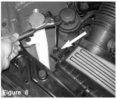
The second m6 bolt located by the wheel welll is loosened and removed from the air box cleaner.
