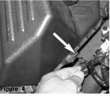
Remove the plastic cliip holding the harness to the side of the air box cleaner.
