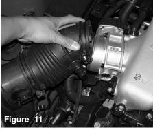
The air intake duct is pulled off of the throttle body as shown above.
