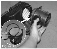
Once you have removed the bolts, continue to detach the mass air flow sensor. Remove the ring from the sensor.
