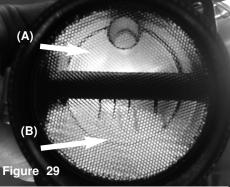
A) As the air fusion tube is inserted into the mass air flow sensor, the tube is placed on the UN-METERED SIDE of the MAF sensor. B)The sensor filaments are shown above.
