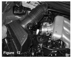
The entire air box and air duct is now ready to be pulled out of the engine compartment.
