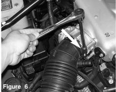
Loosen the clamp on the air intake duct as shown above.
