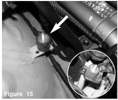
Install the vibra mounts to the factory mounting points of the stock air box.
