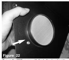
Secure the MAF sensor with the button head inside of the housing. This will allow for maximum clearance for the filter. Tighten using provided M6 nuts.
