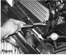
The first bolt in front of the air box cleaner is loosened and removed.
