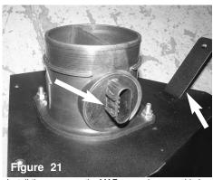
Install the sensor so the MAF sensor harness side is facing the engine. Or also look to see arrow on MAF is facing up and going in the direction towards the throttle body. see step 28.
