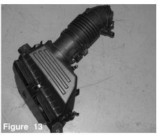
View of the stock air intake box and air intake duct.
