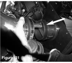
Important: When inserting air fusion tube into the mass air flow sensor step-hose, the air fusion tube MUST BE inserted into the un-metered side
