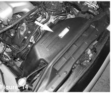
Leave the factory ram air unit. This will be used in the new intake system.
