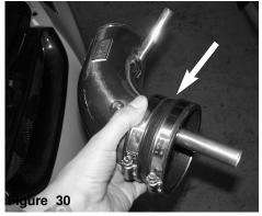
Now install the urethane step hose to the air fusion side of the tube. Tighten the clamp using 8mm nut driver. Install intake assembly into vehicle.
