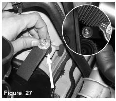
Secure the vibra mounts using provided m6 nuts and fender washers. Tighten using 10mm socket or ratchet
