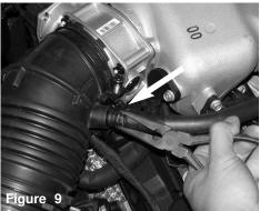
The tension clamp on the crankcase vacuum line is compressed and pulled back, this will allow you to remove the hose from the air duct port.
