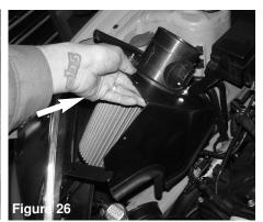
Install the heat shield assembly into the vehicle, position the tabs to the vibra mount.
