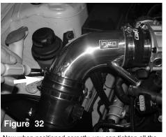
Now when positioned corectly, you can tighten all the clamps using 8mm nut driver.
