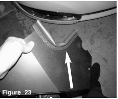
Install the 8" long rubber trim to the cut-out on the heat shield.
