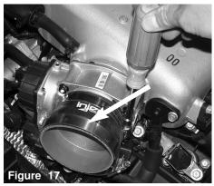
Install the silicon step hose to the Throttle body with clamps provided. Use the smaller clamp on the Throttle body and tighten.
