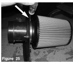
Install the filter to the MAF sensor. Tighten using 8mm nut driver.
