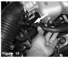
The crankcase vacuum hose is now removed from the air duct port.
