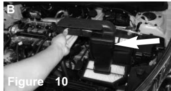
Figure A: Use a phillips screw driver and remove the two plastic screw clips from the front air intake duct Figure B: Lift up and remove the front air intake duct
