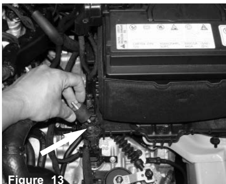
Screw the vibra mount onto the pre-threaded hole next to the battery
