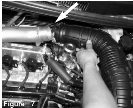
Use a 10mm socket and ratchet and loosen the 10mm clamp bolt on the air duct located on the Turbo charger compressure outlet. Pull the air duct from the outlet.
