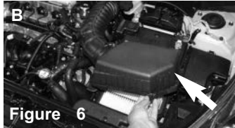
Figure A: Unclip the two tabs from the lower air box assembly to the upper air box assembly. Figure B: Detach the upper air box assembly from the lower assembly
