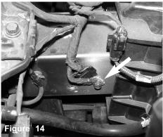
Both wires shown grounded together
