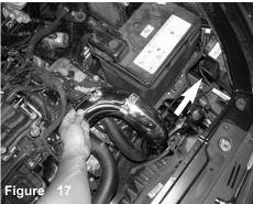
Place the Injen Intake pipe through the chassis In between the battery and headlight in the engine bay. Make sure the end with the two welded nipples are in the engine bay. **NOTE:** Make sure the pipe goes in between the two coolant lines going to the radiator.
