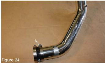
Take the 3" straight hose and press it over the end of the primary intake, use two power-bands and tighten the power-band on the intake side for now.
