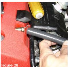
Press the 13"-10mm breather hose over the crank case port as shown above.
