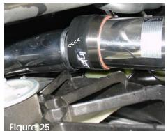
Lower the Primary intake to the side of the radiator fan and insert the 3" hose over the secondary intake.
