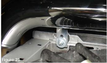
Take the additional m6 flange nut and fender washer and screw them onto the vibra-mount stud to secure the intake.
