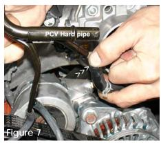
intake port hard pipe on the throttle body line.
