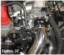
The 13"-10mm hose (A) and air injection pump hose have been installed (B).
