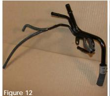
Coolant hard piping removed and replaced with new hoses and coupler.
