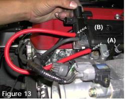
The hose connected to the outside return vacuum port (A) is pressed over the inside port of the VSV (B).
