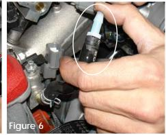
Insert the 6mm coupler into the delivery port hose as shown above. Use stock clamps to secure the coupler in the coolant line
