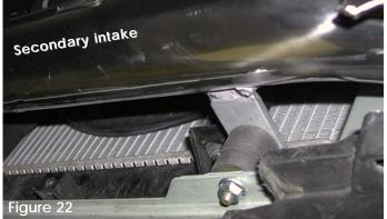
As the filter end is slipped into the bumper cavity, the intake bracket is lined up to sit flush on the vibra-mount stud.
