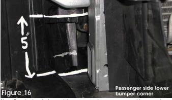
Next, Cut plastic splash guard that separates bumper corner and lower engine bay. A 5" x 5" cut out will be required on the passenger side wall between the front lower engine bay and the front bumper.
