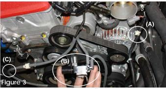
Remove the air intake duct and stock air filter from the lower air box. Unclip the wire harness clip (A), unclip the check valve vacuum line (C) and unscrew the m6 bolt to remove vacuum switching valve (B) all located on the lower air box cleaner. Remove the 3 m6 bolts that secures the lower air box cleaner assembly, then remove the entire lower air box
