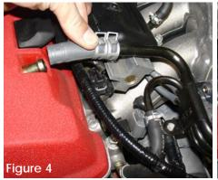
Disconnect the stock breather hose from the crank case port to the hard pipe located over the cam cover.
