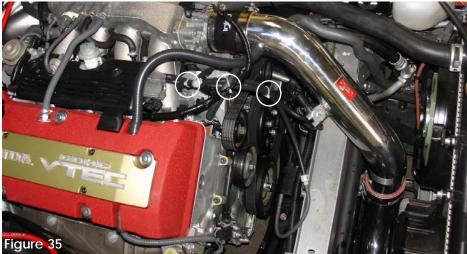
Once the cold air intake has been installed. continue to align the entire intake for best possible fit. Once the intake has been cleared from moving parts or contact from engine components, continue to tighten all nuts, bolts and clamps. Use the three **zip ties** to secure all lines away from moving belts, pulleys and vacuum lines.
