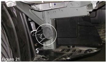
The filter end is inserted into the cut out made earlier and into the bumper cavity.
