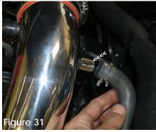
Press the stock air injection pump line over the 3/4" intake port.
