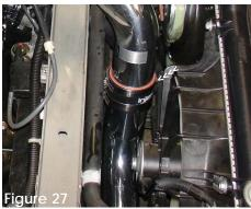
The primary and secondary intakes are butted up together and secured with the two power-bands.
