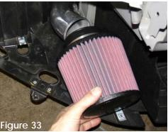
Press the Injen air filter over the end of the secondary intake located in the bumper cavity, continue to tighten filter neck clamp.
