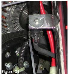
Line up the vacuum switching valve to the intake bracket and use the 5mm bolt to secure it in place. Reconnect harness clip over the vacuum switching valve until it snaps in place.
