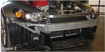
Remove the front bumper (A). Unclip the six clamps on the lid of the air box, then remove the top lid (not shown). 1- Loosen clamp on the throttle body air intake duct, 2- Remove vacuum hard pipe from the crank case to the air intake port and 3- Remove air injection pump hose located on the opposite side of the crank case breather hard pipe.
