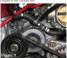
Use the stock clamps to secure the coolant lines to the coupler.
