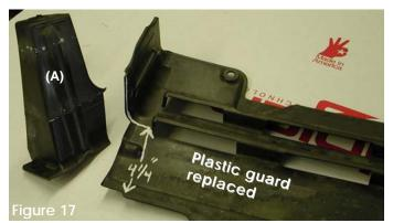
Remove the bottom splash guard located underneath the engine, between the wheels. Cut the plastic leg that attaches on the passenger side(A). Once the plastic leg has been cut out, continue to re-attach the splash guard again.
