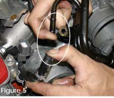
PCV hard pipe removed: Disconnect Coolant delivery port to the side of the engine block leading to the throttle body coolant intake port.
