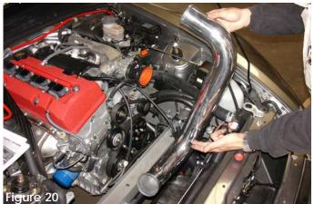
The secondary intake is now lowered into the position across the bottom edge of the radiator.
