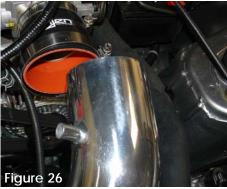
Insert the top end of the primary intake into the throttle body hose.
