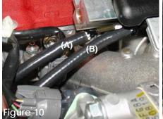
Remove stock exhaust and return vacuum lines then continue to install the Two 16"-4mm vacuum hoses provided. Press one hose over the exhaust vacuum port(A) and press the other over the return vacuum port (B). Page 2 of Part # SP1305
