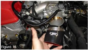
Press the silicone step hose over the throttle body and use two powerbands. Tighten the power-band located on the throttle body side at this time.
