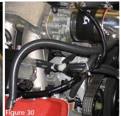
The 13" -10mm hose has been connected to the crank case port and the intake port.
