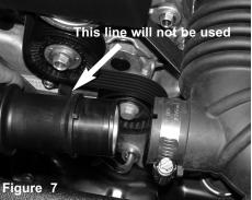
Loosen the clamp on the intake tube and remove the sound tube. This will no longer be used on the new Injen intake system.
