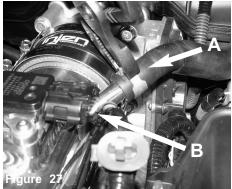
A)Secure the crank case line to fitting on tube using
