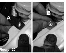
A) Place provided hex screw from bottom of radiator support through tab. Hold screw in place.
