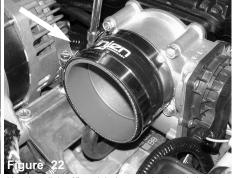
Now install the 3" straight hose to the throttle body with clamps and tighten on the throttle body only.
