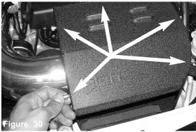
With provided M6 button head screws, secure the cover and tighten. Re-position if necessary. <u>NOW CONNECT BATTERY TERMI-</u> NALS. START VEHICLE AND LET IDLE FOR 5 MINUTES.
