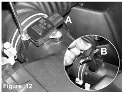
A)Loosen the 2 screws holding in the MAF sensor using Install the MAF sensor into the intake tube. the phillips screwdriver. B)Remove the MAF sensor from the vehicle.
