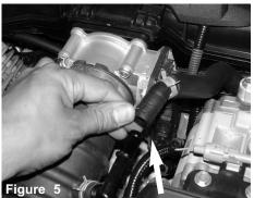
With pliers, pull back the crank case line from the intake fitting.
