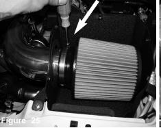
Install the filter to the intake tube and tighten using 8mm nut driver. MAKE SURE THAT THE FILTER FLANGE GOES ON THE TUBE 3/4"-1" AND STOP. DO NOT FORCE FILTER ON ANY FURTHER.
