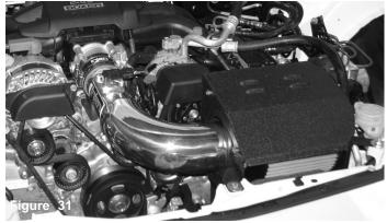
Congratulations! You have just completed the installation of this intake system. Periodically, check the alignment of the intake, normal wear and tear can cause nuts and bolts to come loose. <u>Note: Check clearance and adjust if needed!</u> Failure to check the alignment and adjust the intake can cause damage that will void the warranty. Injen Technology is not responsible for any damages caused by/from improper installation.
