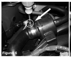
Loosen the clamp on the Sound Tube resonator.
