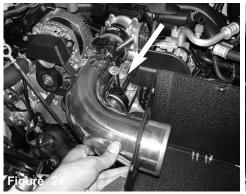
Position for best fit. *Tube will have slight angle for filter to clear heat shield cover. Make sure the tube sits up against the throttle body. Do not tighten.*
