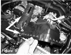
Un-clip the upper part of the air box, remove the upper assembly including the intake tube from the vehicle.
