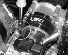
Now position for best fit, Secure and tighten using 8mm nut driver.
