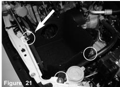
Tighten all screws using 10mm socket and ratchet.
