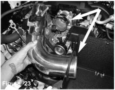
Now install intake tube through heat shield and position to throttle body.
