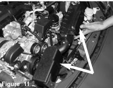
Now lift up and remove the lower intake assembly from vehicle.
