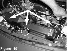
Loosen the 3 bolts holding in the bottom half of the air box using 10mm socket and ratchet.
