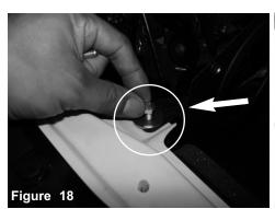
Secure the front of the heat shield using provided M6 hex screw and fender washer.
