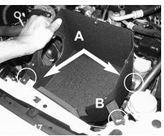
A)Install the heat shield and position the tabs to factory mounting points. B)Position tab to radiator support from step 15.
