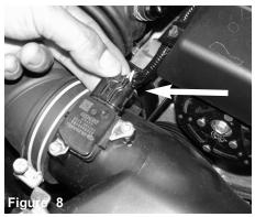
Disconnect MAF sensor harness and pull line away from air box.
