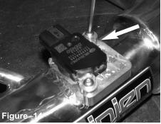
Secure MAF sensor using provided M4 button head screws. Tighten using 2.5mm allen key.
