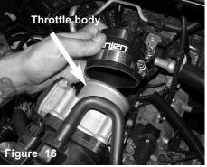
Install the 2-3/4" straight hose with clamps to the throttle body. Tighten clamp on throttle body only.
