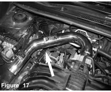
Install the upper intake tube and position to the hose on throttle body. Do not tighten.
