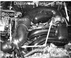
Disconnect the MAF sensor harness, crankcase line and the two clamps on the factory intake air duct.
