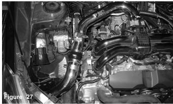
Check the entire system for the best possible fit. Once you have checked the entire system for leaks, rubbing or rattling, continue to tighten all nuts, bolts and clamps. Reconnect the negative battery terminal prior to starting the engine.
