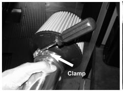
Attach the filter to the lower intake assembly. Tighten using 8mm nut driver.
