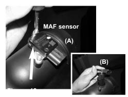
A) Loosen the 2 screws holding in the MAF sensor using phillips screwdriver. B) Remove the MAF sensor from the air box.
