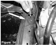
locate the threaded insert on frame and install and tighten.
