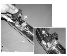
A) Install the MAF sensor into the intake tube. B) Secure using provided M4 screws and tighten.
