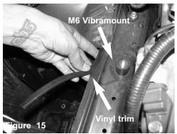
Secure the vibramount and tighten. Attach a vinyl trim to the edge of the vehicle frame.
