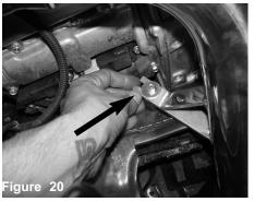
Position for best fit, Do not tighten clamps. Secure the bracket using provided fender washer and nut.
