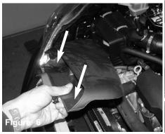
Remove the two plastic retaining clips indicated by the Unclip the metal retaining clips top air box and arrows and then remove the front air scoop.
