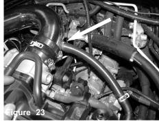
Secure the 12mm hose to the fitting on intake tube.
