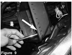
With extension and 10mm socket, inside of air box loosen the 10mm nut holding in the remaining half of air box.
