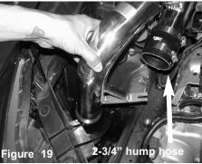
Attach the 2-3/4" hump hose with clamps to the upper intake tube assembly. Install the lower intake assembly into vehicle. Positon bracket to the vibramount
