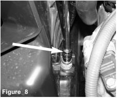
Loosen the screw holding in the air box.
