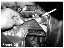
Position for best fit and tighten all clamps using 8mm nut driver. Tighten the vibramount using 10mm wrench.
