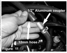
Locate the crankcase line. Insert the provided 1/2" aluminum coupler and secure. now install and attach the provided 12mm hose to the aluminum coupler.
