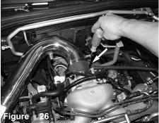
Tighten clamp using 8mm nut driver.
