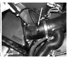
With phillips loosen the 2 screws that hold in MAF sensor.
