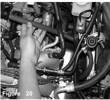
Attach the new provided 10mm crank case line to engine and position to new vehicle.
