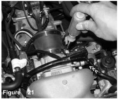
Install new step hose with clamps to throttle body and tighten on throttle body only.
