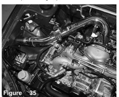
Align the entire intake for the best possible fit. Once you have cleared the intake from all moving parts, continue to tighten all nuts, bolts and clamps.
