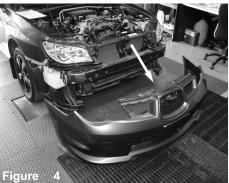
Remove the 9 plastic push clips on bottom of bumper. Remove bumper.
