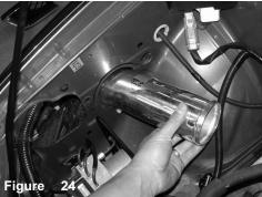
Install cold air unit through cut out.
