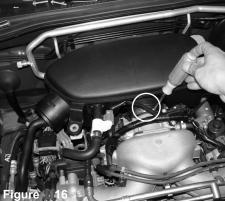
With 8mm nut driver, loosen the clamp holding in plenum box on throttle body.
