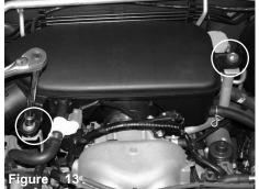
With 10mm socket and extension, loosent he 2 bolts holding in plenum box.
