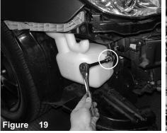
Loosen the remaing bolt on noise box on frame of vehicle. Remove the noise box from vehicle.
