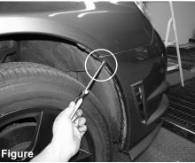
Remove the plastic cip on both sides of bumper
