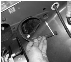
Attach the vinyl trim to hole cut out on inside of fender well.
