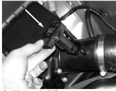
Carefully remove the MAF sensor.
