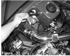
Tighten all clamps on silicon elbow hose in both images using 8mm nut driver. Once you have aligned and tightened all nuts, bolts and clamps, continue to install the front bumper to its original position.
