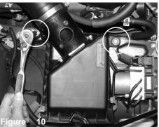
With 8mm nut driver, loosen the clamp on plenum box. With 12mm socket and extension, loosen the 2 bolts that hold in stock air box.
