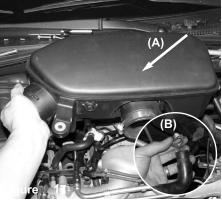
A)Carefully pull up and remove plenum box.
