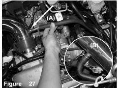
A) Attach crank case line to intake tube.
