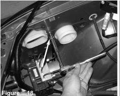
Loosen the bolt holding in plastic noise box from inside of engine compartment on fender using 10mm socket with ratchet.
