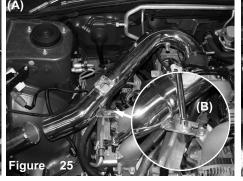
A) Install upper intake and position to throttle body and bracket to vibra mount. B) Secure the bracket using washer and M6 nut.
