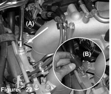
A) With 12mm socket loosen the bolt holding in bracket and remove. B) Replace and secure with M6 vibra mount.
