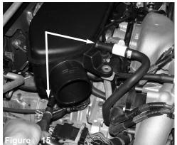
Pull back any vacuum lines from plenum box. 2005 model only should have 1 vacuum line.
