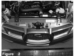
Removal of front bumper is required. Remove the 6 big plastic clips, 4 small clips on grill on top. Remove both using phillips. front grills.
