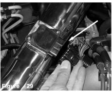
Install straight hose with clamps and connect the cold air tube to upper intake tube.
