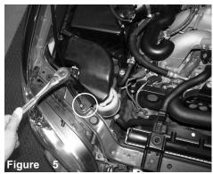
Loosen and remove intake scoop from core support.
