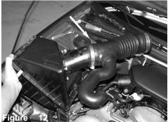
Carefully pull out stock air box out of vehicle.
