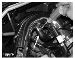
06-07 models, using provided mini clamp, secure vacuum line to fitting on intake tube and tighten.
