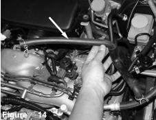
Remove the crank case from engine and plenum box.
