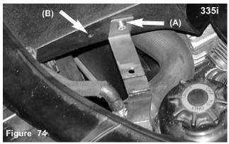
The bracket on the 335i is now installed as shown above (A). Note: On the 335i, the bracket is secured on the second press nut. If used on the 135i, the bracket is fastened to the first press nut (B).
