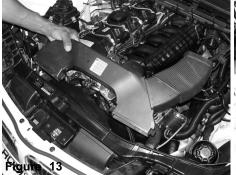
Once all four bolts have been removed, continue to pull the air scoop duct out.
