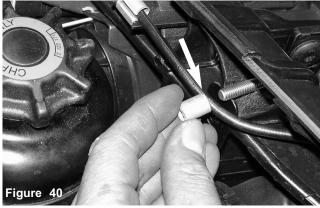
The 3/16" aluminum spacer is slipped over the m6 x 35mm bolt used to secure the reservoir bracket. **NOTE: Spacer is only required on the 135i**
