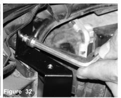
An allen wrench is used to tighten the 35mm bolt into the head lamp pre-tapped hole.
