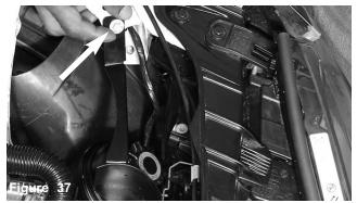
The stock m6 bolt is used to fasten the extended bracket located on the new power steering cup.
