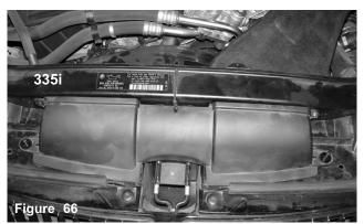
The front air scoop is now installed in the 335i.
