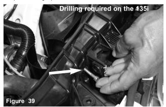
Insert the m6 x 35mm hex bolt through the composite cross member and through the 3/8" aluminum coupler as shown in figure 26.
