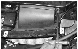
Attaching the Injen air scoop to the 135i: The m6 x 16mm bolts are used to attach the stock front air scoop to the new engine air scoop. Page 8 of Part# SP1125
