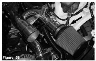
Once the intake end has butted up against the filter stops, continue to tighten the filter clamp.
