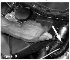
The clamp on the front air box inlet is now loosened.
