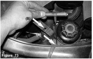
The allen wrench is now used to fasten the bolt tight (A). If you choose to use the bracket on the 135i, the upper hole is aligned to the reservoir bracket (B).
