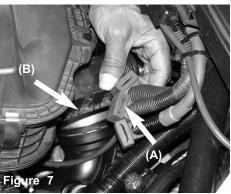
The harness rubber hangers have been removed from the prongs on the air box inlet(A). The inlet on the air box has also been separated (B).
