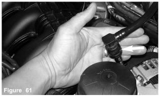
The brake vacuum hard line is pressed over the lower female hard line. Do not attempt to drive vehicle until this line has been reconnected.
