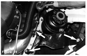
Remove the both m6 nuts from the lower power steering brace(A) and the 10mm flange bolt from the edge of the fender well(B).
