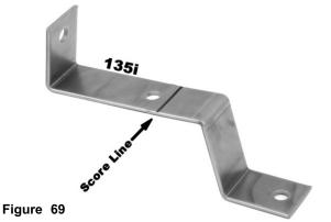
When attaching the bracket shown above, the 335i uses the entire bracket shown above. Using the bracket on 135i is optional, if you opt to use the bracket, break or cut bracket at the score line as shown above.
