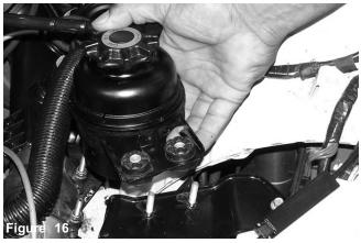
Once both m6 nuts have been removed, continue to pull the power steering reservoir from the two studs.
