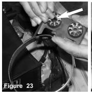
The aluminum stud is removed from one of the grommets.
