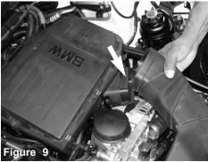
Pull the air scoop inlet from the air box inlet as shown above.
