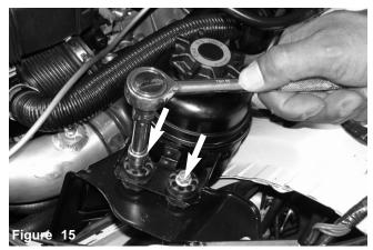
Loosen and remove both m6 nuts from the power steering brace.
