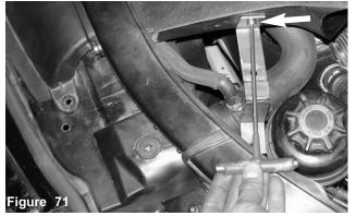
An allen wrench is used to fasten the bolt to the air scoop nut insert.
