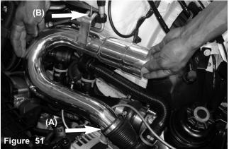
The U-bent intake is lowered into the engine compartment. The lower end is inserted into the air intake duct (A) and the upper bracket is aligned to the vibra-mount stud (B). Page 6 of Part# SP1125
