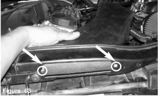
Both hole patterns will line up to the pre-drilled holes on the 135i, use two m6 x 16mm bolts to fasten the air scoop. The 335i will only take one bolt on the air scoop, the scoop bracket will be used to strengthen and attach the air scoop to the reservoir bracket.
