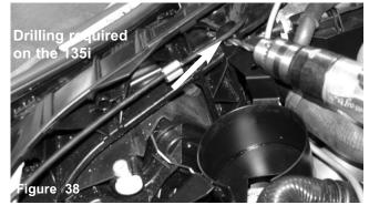
Applicable to the 135i only: Use a 1/4" drill bit to drill a hole through the composite cross member, the short bracket on the cup is used as a pattern.
