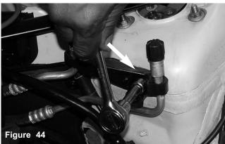
Remove the 10mm nut that holds the air conditioning lines to the side of the tower mount as shown above.
