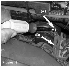
The clamp on the rear air inlet is loosened (A) Note: position of harness rubber hangers (B).
