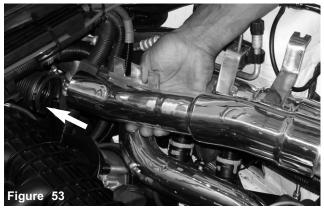
The step down intake is lowered into the engine compartment and pressed into the rear air intake duct.
