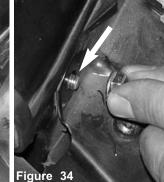
Once you have inserted the 35mm bolt all the way in, continue to place the m6 flange nut over the bolt end.
