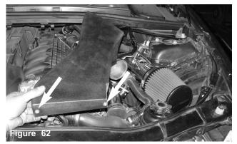
The air scoop is lowered into the engine compartment, The press nuts are aligned to the cross member pre-drilled holes.
