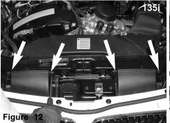
Loosen and remove the four bolts holding the primary air scoops in place.
