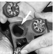
The grommet is now pulled from the metal brace.
