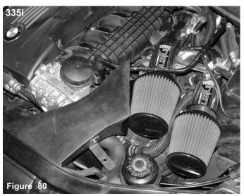
Congratulations! You have just completed the installation of this intake system. Periodically, check the alignment of the intake, normal wear and tear can cause nuts and bolts to come loose. Failure to check the alignment and adjust the intake can cause damage that will void the warranty.
