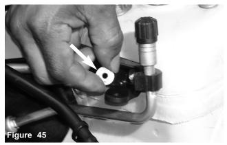
The two m6 nuts is loosened and removed from the threaded stud supporting the hard line and brace.
