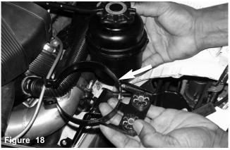
Once you have removed the m6 bolt, continue to remove the clamp from the power steering reservoir bottle.
