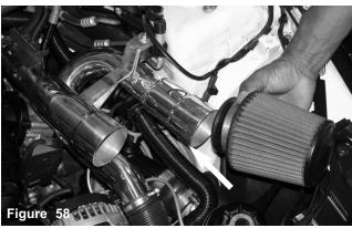
The first filter is aligned and pressed over the U-bent air intake.
