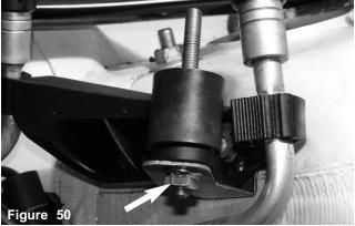
The m6 flange nut is now tightened to keep the vibra-mount from slipping out of the bracket.
