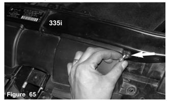
Attaching the air scoop to the 335i: The front scoop is re-attached to the cross member and the stock bolt is used to fasten the front scoop to the new engine air scoop. The plastic clips are also used on the scoop.
