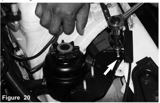
Loosen and remove the m6 bolt from the upper brace as shown above.
