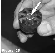
The aluminum stud is installed in the the stock grommet.
