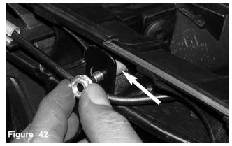
The m6 flange nut is used to tighten the reservoir bracket in place. **Note:** The 3/16" spacer between the bracket and cross member, used to support the bracket to keep it from distorting.
