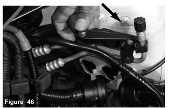
The brace is now pulled from the tower mount threaded stud as shown above. This will allow a space between the fender well and the brace.
