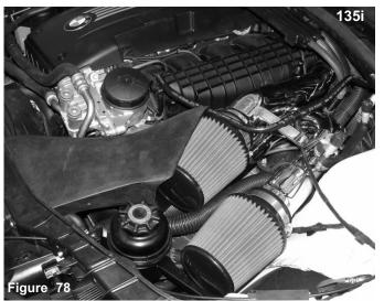
Note: The secondary filter on the 135i will fit snug inside of the air scoop as shown above. The secondary filter will have space around the filter when installed in the 335i.
