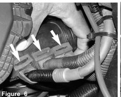
Rubber hangers are lifted from the prongs located on the air box inlet.
