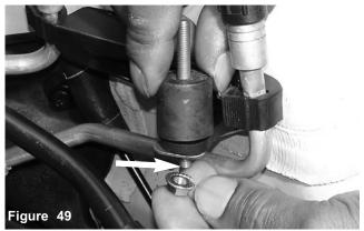
The vibra-mount is inserted into the new stainless steel bracket and the m6 flange nut is aligned to the vibra-mount stud.
