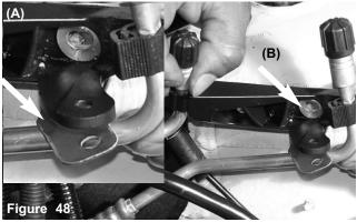
The new stainless steel Injen bracket is matched up to the composite brace. The assembled braces are placed on the threaded stud and fastened and fastened with the stock m6 flange nut (B).
