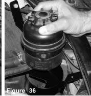
Once you have installed the reservoir cup in place, continue to lower the power-steering bottle in place.
