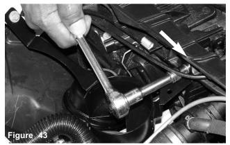
A 10mm socket and ratchet is used to fasten the flange nut to the m6 bolt.
