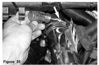
Once the intake has been aligned, continue to tighten the air duct clamp.
