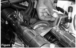
Once the intake has been inserted into the air intake duct, the intake bracket is aligned to the vibra-mount stud.
