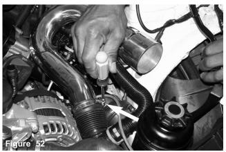
The air duct clamp is tightened as shown above.
