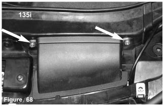
The stock air scoop is now attached to the new Injen air scoop.
