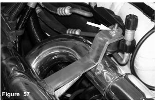
The m6 flange nut and fender washer is used to fasten the secondary intake to the vibra-mount stud.
