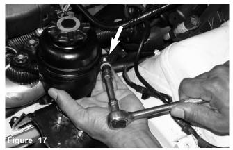
Remove the m6 bolt from the power steering clamp.
