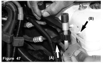
The new stainless steel bracket is placed under the plastic stock bracket(A) while placing the bracket over the threaded stud and tower mount(B).
