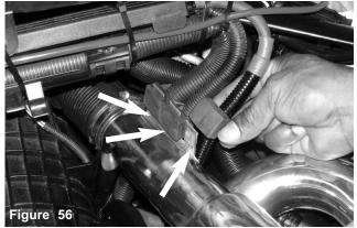
The three rubber harness hangers are pressed over the aluminum prongs located on the air intake as shown above.
