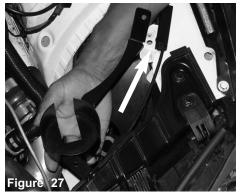
The reservoir cup is lowered into the engine compartment. The long cup bracket is aligned to the fender wall brace.
