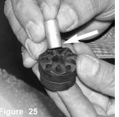
The aluminum stud in pressed into the grommet.
