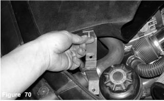
An m6 x 10mm bolt is used to attach the upper bracket to the second nut insert located on the air scoop.
