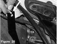
The stock m6 bolt is screwed into the pre-tapped hole.
