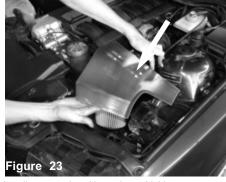
Install cover and position to heat shield.
