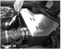
Make sure that the cable line is through the cut out on cover and heat shield.
