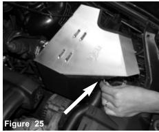
Secure the cover using the provided stainless M6 screws.
