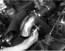
Position for the best fit and secure the bracket using provided washer and nut. Tighten using 10mm socket or wrench.
