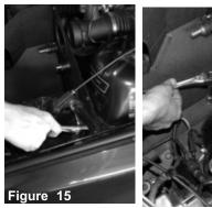
A&B) Tighten and secure heat shield using the 10mm socket and ratchet.
