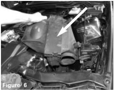
Carefully lift up and pull out the air box.
