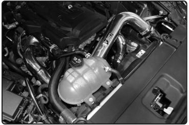
Congratulations! You have just completed the installation of this intercooler pipe system. Periodically, check the alignment of the intake, normal wear and tear can cause nuts and bolts to come loose. <u>Note: Check clearance and adjust if needed! Failure to</u> check the alignment and adjust the intake can cause damage that will void the warranty. Injen Technology is not re-sponsible for any damages caused by/from improper installation.
