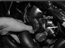
**10.** Pull back the intercooler pipe from turbo.
