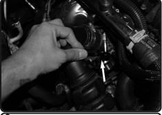
**8.** Loosen the clamp on the turbo for the hot side of the intercooler pipe using 7mm nut driver or ratchet. Loosen the clamp on the intercooler side also. Page 3 SES9200ICP
