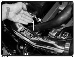
**16.** Secure the bracket using provided M6 nut and fender washer.
