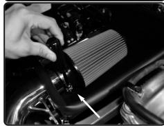
**19.** Tighten filter using 8mm nut driver.
