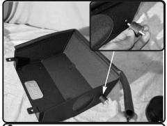
**6.** Install the provided rubber trim to the top of the heat shield. Notch corners for easy installation with pliers. Install the m6 vibramount to the thredded insert on heat shield.
