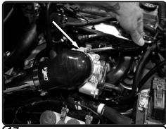
17. Now position the intake tube for best fit, close hood to see the cobrahead is in the correct position and does not hit. Tighten both clamps using 8mm nut driver.
