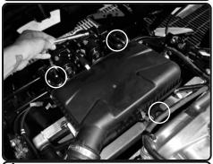
**4.** With 10mm socket and extension and ratchet, loosen the 3 bolts holding in the air box.
