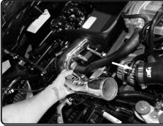
**15.** Now install intake tube and position the tube through heat shield and bracket to vibramount on heat shield. Install to cobra head, Do not tighten.
