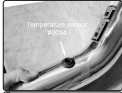
7. Install the temperature sensor grommet to the hole on intake tube.
