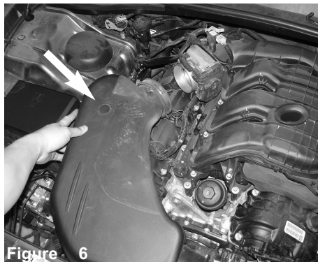
Figure 6 Remove the air duct from the throttle body.
