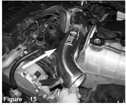
Install the intake tube and position to the elbow coupler and the bracket to the vibra mount.
