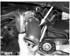
Install the elbow with clamps provided to the throttle body. Make sure the 2-3/4" side is installed on the throttle body.
