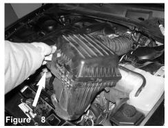
Now lift up and remove the complete stock intake system.
