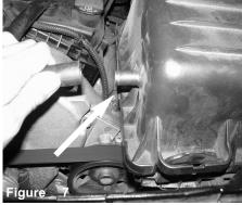
Pull back the crank case line from the stock air box.
