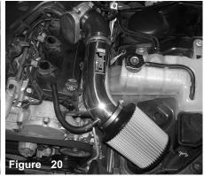
Align the entire intake for the best possible fit. Once you have rechecked and cleared the intake from all moving parts, continue to tighten all nuts, bolts and clamps.
