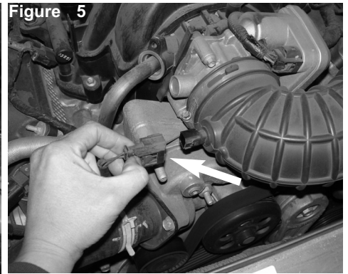
Once the engine cover is remove, disconnect the harness from the air temperature sensor
