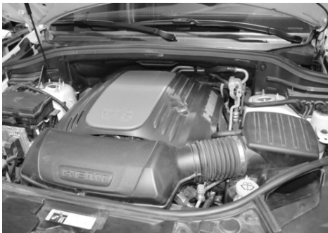
Figure 2 Complete stock air intake cleaner and air intake duct.
