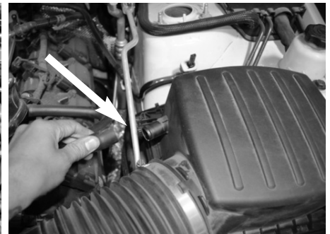
Figure 4 Pull back the crank case line from the air box.
