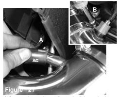
A)Connect the crank case line to the fitting on intake tube. B) Tighten the clamp on throttle body and connect the temperature sensor harness.
