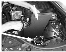
Install the heat shield assembly into the vehicle and position the tabs to the vibra mounts.
