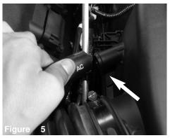
Pull back the crank case line from the air box fitting.
