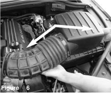
Remove the complete air box assembly out of the vehicle.
