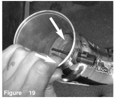
Install the temperature sensor into the intake tube and secure.
