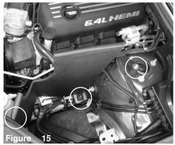
Secure the heat shield using provided M6 nuts and fend-
