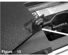
Install the heat shield grommet to the tab located at the bottom of the heat shield. Note: this will seat into the factory fitting of stock air box.
