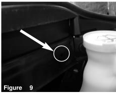
Locate the hole that is on the radiator support behind the washer resovoir filler.
