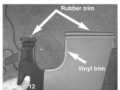
Install the rubber trim to the top of the heat shield. Install the vinyl trim to the cut out on the heat shield.
