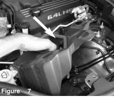
Remove the plastic air box splash guard.
