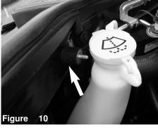
Install the male/male vibra mount secure the back of the vibramount using provided m6 nut.
