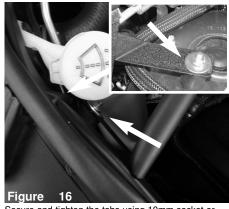
Secure and tighten the tabs using 10mm socket or wrench.
