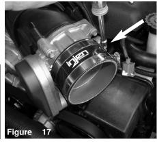
Install the straight hose with clamps to the throttle body. Tighten the clamp on throttle body using 8mm nut driver.
