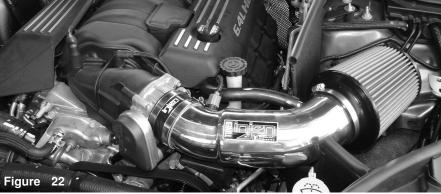
Install the air fitler and tighten using 8mm nut driver. Congratulations! You have just completed the installation of this intake system. Periodically, check the alignment of the intake, normal wear and tear can cause nuts and bolts to come loose. Note: Check clearance and adjust if needed! Failure to check the alignment and adjust the intake can cause damage that will void the warranty. Injen Technology is not responsible for any damages caused by/from improper installation.
