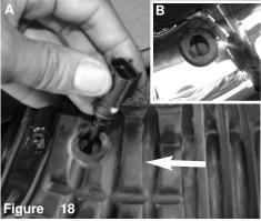
A) Remove the temp sensor from the stock intake tube. B) Install the temp sensor to the hole on intake tube.
