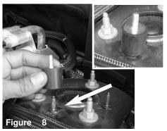
Locate the M6 thredded fitting on the strut tower and secure the male/female vibra mount.
