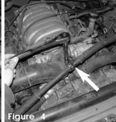
Now loosen the 10mm bolt on the power steering hose bracket attaching it to the air duct.
