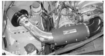
Press the 31/2" Injen filter over the end of the intake. Adjust the filter for best fit and tighten the clamp on the filter neck. Screw the additional m6 x 20 hex head screws into the remaining press in nuts
