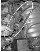
Remove the vacuum switching valve line from the back side of the air duct. (Figure A). The entire vacuum switching valve line is remove and will be replaced with an Injen vauum line later. (Figure B)
