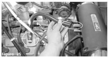
Take the 15mm hose connected at the crankcase port and press it over the 5/8" port located on the intake.
