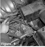
Now disconnect the crank case vacuum line from the valve cover to the vacuum box on the air duct.
