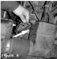
Disconnect the vacuum line connected to the side of the air duct.
