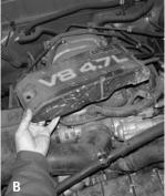
Use a 10mm socket and rachet and remove the two 10mm nut holding down the engine cover. (Figure A) Then remove the engine cover to get to the clamp on the intake duct. (Figure B)
