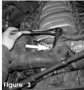
Use a 10mm socket and rachet and loosen the 10mm clamp on the intake duct at the throttle body.
