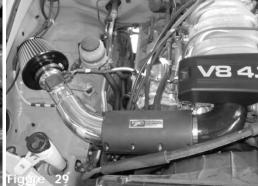
Align the entire intake for best fit. Check all vacuum lines for any leaks. Once all lines and fit has been checked continue to tighten all nuts, bolts and clamps.
