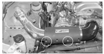
Press the assembled heat shield and intake and insert the straight end into the elbow located on the throttle body. Align the intake while pressing it into the elbow but be sure to align the bracket to the vibra-mount stud. You may loosen the heat shield screws to further adjust the shield.
