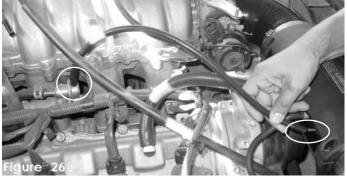
Take the 4mm vacuum hose connected to the pressure regulator port and insert it over the 3/16" vacuum port located on the intake.
