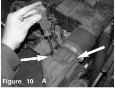
Use a phillips to unscrew the two screws holding down the MAF sensor. (Figure A) Then remove the MAF sensor from the factory air box cleaner
