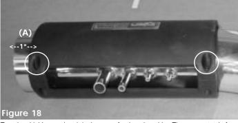
Turn the shield around and do the same for the other side. There are a total of four m6 x m25 hex screws used to attach this heat shield. Do not over tighten the screws because minor adjusting will be required to set the heat shield in the correct location. Allow at least 3/4" to 1" from the end for the 90 degree elbow (A).
