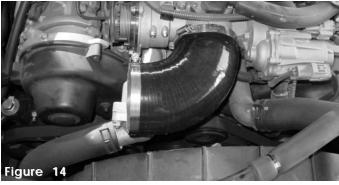
Press the 3 1/4" end on the 90 degree elbow over the throttle body. Place a clamp on each side of the elbow but only tighten the end on the throttle body.
