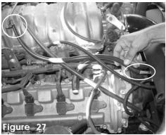
All 2000-02 will have a charcoal canisters with vacuum port. Take the 8mm hose connected to the charcoal canister and press it over the 3/8" port on the intake.
