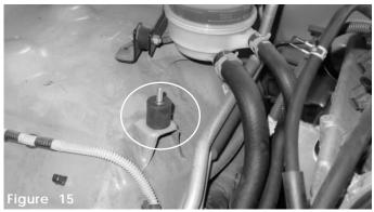
Screw the grey vibra-mount into the brace located on the the fender well until it bottoms out.
