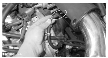
Take the stock power steering vacuum line and press it over the 1/4" port located on the intake
