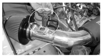
Remove the stock mass air flow sensor from the stock intake box. Press the sensor into the machined adapter located on the intake. It is good practice to wet the O-ring with a dab of water or oil in order to prevent the O-ring from kinking or tearing as it is pressed in.
